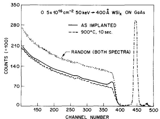
Fig. 1. Ion-channelling spectra before and after annealing (900 °C, 10 s) from a 400 Å  $\text{WSi}_{0.45}$ -GaAs sample implanted with oxygen ( $5 \times 10^{16} \text{ cm}^{-2}$ , 50 keV).
