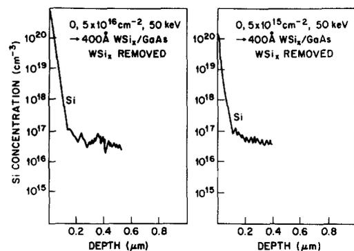
Fig. 5. SIMS profiles of silicon knocked into GaAs by through-implantation of 400 Å of  $\text{WSi}_{0.45}$  on the GaAs surface by 50 keV  $\text{O}^+$  ions at doses of  $5 \times 10^{16} \text{ cm}^{-2}$  (left) and  $5 \times 10^{15} \text{ cm}^{-2}$  (right).
