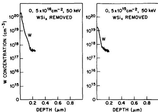
Fig. 4. SIMS profiles of tungsten knocked into GaAs by through-implantation of 400 Å of  $\text{WSi}_{0.45}$  on the GaAs surface by 50 keV  $\text{O}^+$  ions at doses of  $5 \times 10^{16} \text{ cm}^{-2}$  (left) and  $5 \times 10^{15} \text{ cm}^{-2}$  (right).
