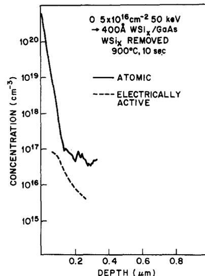
Fig. 6. Atomic and electrically active profiles of silicon in GaAs after through-implantation of 400 Å of  $\text{WSi}_{0.45}$  on the GaAs surface by 50 keV  $\text{O}^+$  ions at a dose of  $5 \times 10^{16} \text{ cm}^{-2}$  and subsequent annealing (900°C, 10 s).
