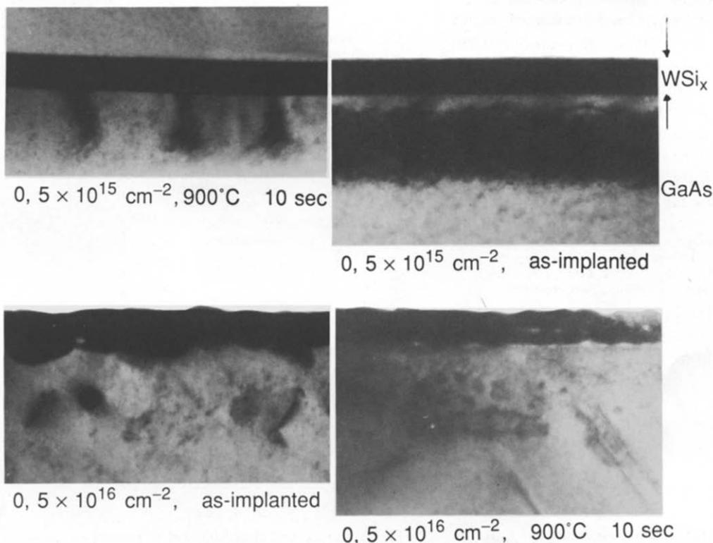
Fig. 2. TEM cross-sections from  $400 \text{ \AA}$   $\text{WSi}_{0.45}$ -GaAs samples after implantation with oxygen at  $5 \times 10^{15} \text{ cm}^{-2}$  (top left) and  $5 \times 10^{16} \text{ cm}^{-2}$  (bottom left), and after subsequent annealing at  $900^{\circ}\text{C}$  for 10 s (top right and bottom right respectively).
