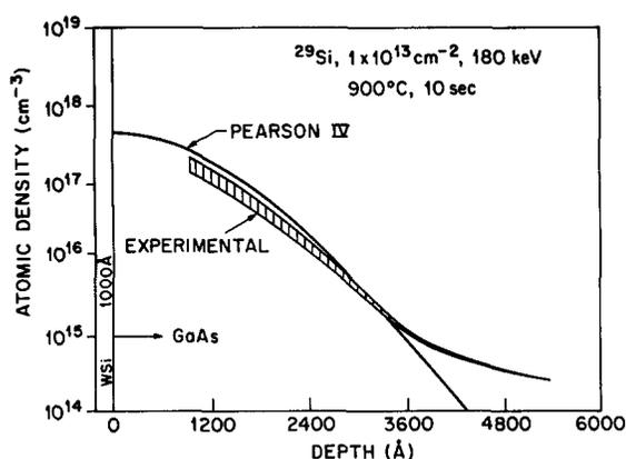
Fig. 7. Theoretical and experimental carrier profiles in GaAs after through-implantation of 1000 Å of  $\text{WSi}_{0.45}$  on the GaAs surface with silicon ( $1 \times 10^{13} \text{ cm}^{-2}$ , 180 keV) and subsequent annealing at 900°C for 10 s. The shaded region represents the range of carrier profiles measured at 12 spots over a wafer 2 inches in diameter. The Pearson IV distribution is the theoretically predicted ion distribution.
