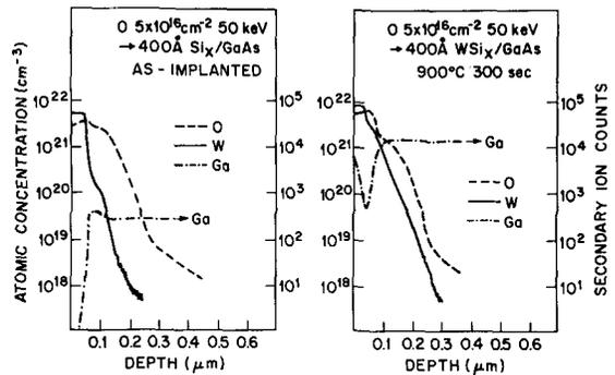
Fig. 3. SIMS atomic profiles of oxygen, tungsten and gallium in  $400 \text{ \AA}$  in  $\text{WSi}_{0.45}$ -GaAs samples implanted with oxygen ( $5 \times 10^{16} \text{ cm}^{-2}$ , 100 keV), before and after annealing at  $900^{\circ}\text{C}$  for 10 s.
