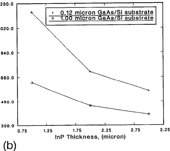
FIG. 1. Crystal properties of 3  $\mu\text{m}$  InP on 1  $\mu\text{m}$  GaAs/Si substrates. (a) X-ray diffraction rocking curve, (b) variation of rocking curve linewidth with GaAs/Si and epitaxial InP thicknesses.
