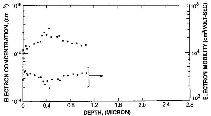
FIG. 2. Electron mobility and concentration profiles of InP-on-Si at 300 K as determined from differential Hall measurements.
