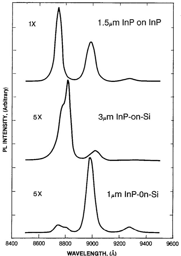
FIG. 3. Photoluminescence spectra of InP-on-Si at 10 K.
