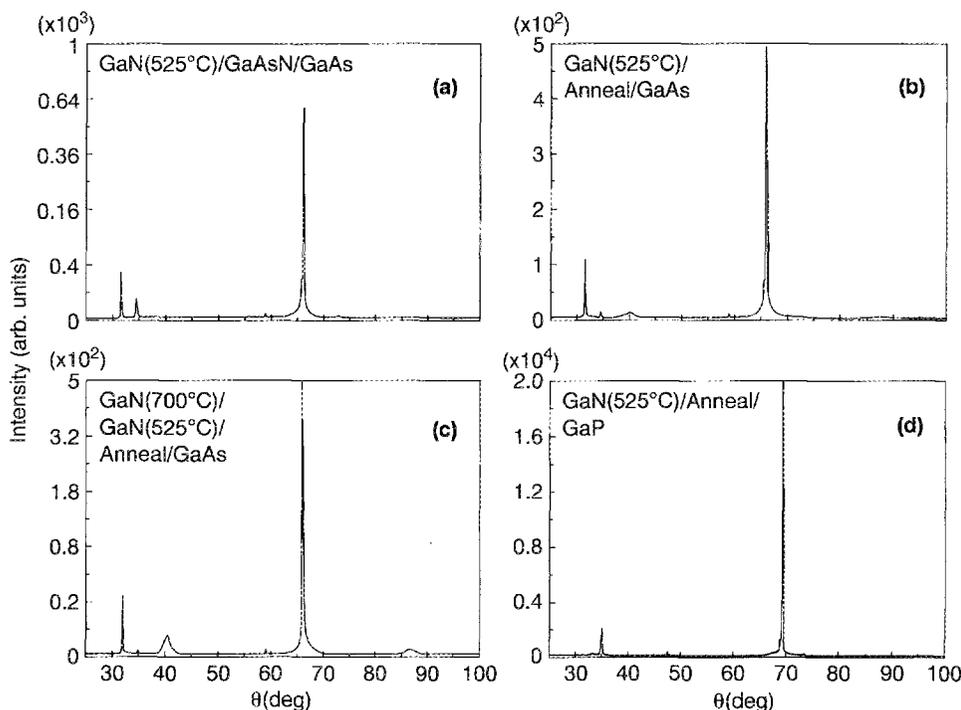
FIG. 3. XRD scans of GaN grown on either GaAs (a)–(c) or GaP (d). Scan in (a) was taken from a sample with a graded GaAs<sub>x</sub>N<sub>1-x</sub> buffer while the other samples were grown with a 15 min *in situ* anneal under a nitrogen plasma. Samples depicted in (a), (b), and (d) were deposited at 525 °C. The layer shown in (c) was deposited at 700 °C after deposition of a thin, ~500 Å, GaN buffer layer at 525 °C.
