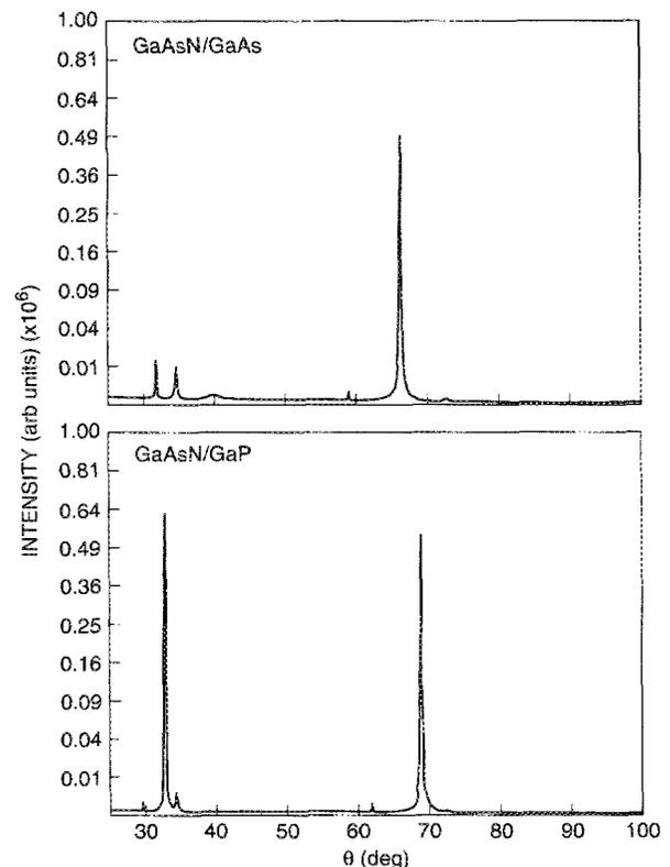
FIG. 2. XRD scans of GaAs<sub>x</sub>N<sub>1-x</sub> grown at 700 °C on GaAs (top) and GaP (bottom).
