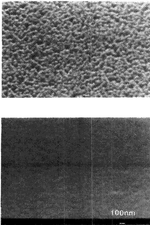
FIG. 1. SEM micrographs of GaAs<sub>x</sub>N<sub>1-x</sub> grown at 700 °C on GaAs (top) and GaP (bottom).
