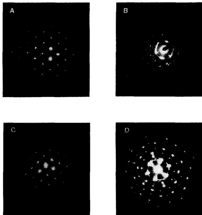
FIG. 4. SADP of GaN layers grown at 700 °C (b) or 525 °C (a), (c), and (d) on GaAs (b) and (d) or GaP (a) and (c). Pattern depicted in (a) was taken in the bulk while (c) was taken at the film/substrate interface.
