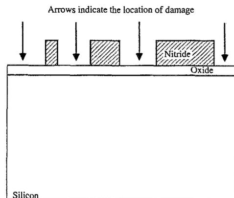
FIG. 1. Cross section of the wafer showing the stripe structures used in the experiment.
