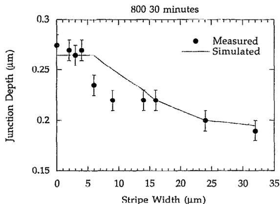
FIG. 2. Measured and simulated junction depths as a function of the stripe width.
