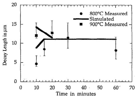
FIG. 3. Extracted decay length from measurement and simulation as a function of anneal time and temperature.
