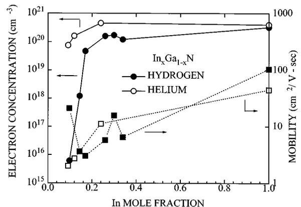
FIG. 1. Electron concentration and mobility at 300 K in  $\text{In}_x\text{Ga}_{1-x}\text{N}$  films grown at  $500^\circ\text{C}$  on GaAs as a function of ternary composition.
