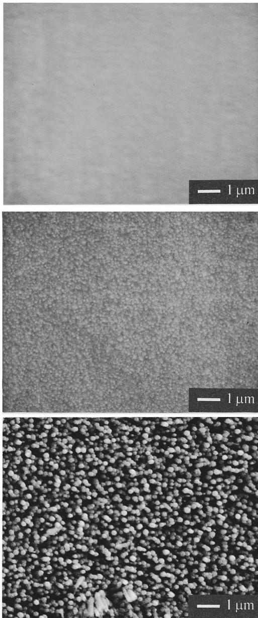
FIG. 2. SEM micrographs of InGaN films. Ga mole fraction increases from (top) 0.33 to (center)  $\sim 0.53$  to (bottom)  $\sim 0.64$ . Layers were grown on GaAs at 500 °C using the same TMI flow rates.
