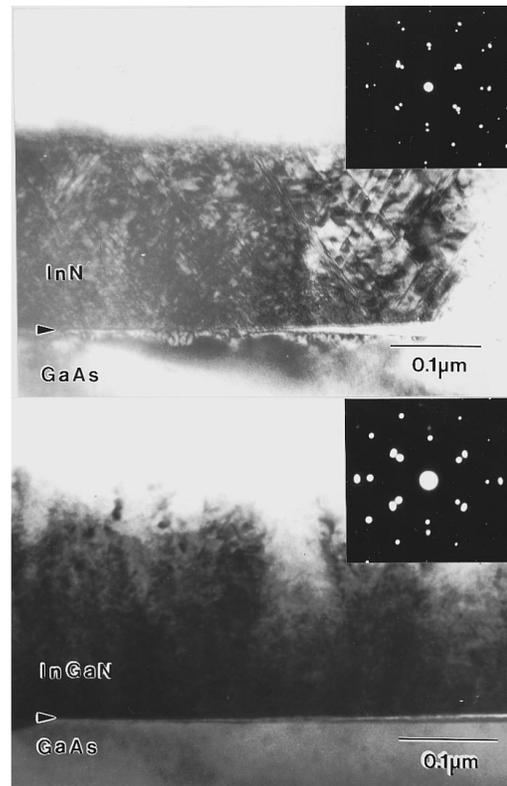
FIG. 3. Cross-section TEM micrographs and selected area diffraction patterns from InN (top) and  $\text{In}_{0.26}\text{Ga}_{0.74}\text{N}$  (bottom) samples grown directly on GaAs. The TEM was performed under bright-field,  $g=[220]$  conditions.
