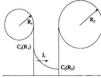
Fig. 7. Schematic diagram to illustrate the Si self-interstitial concentration gradient established due to the size difference of the dislocation loops.
