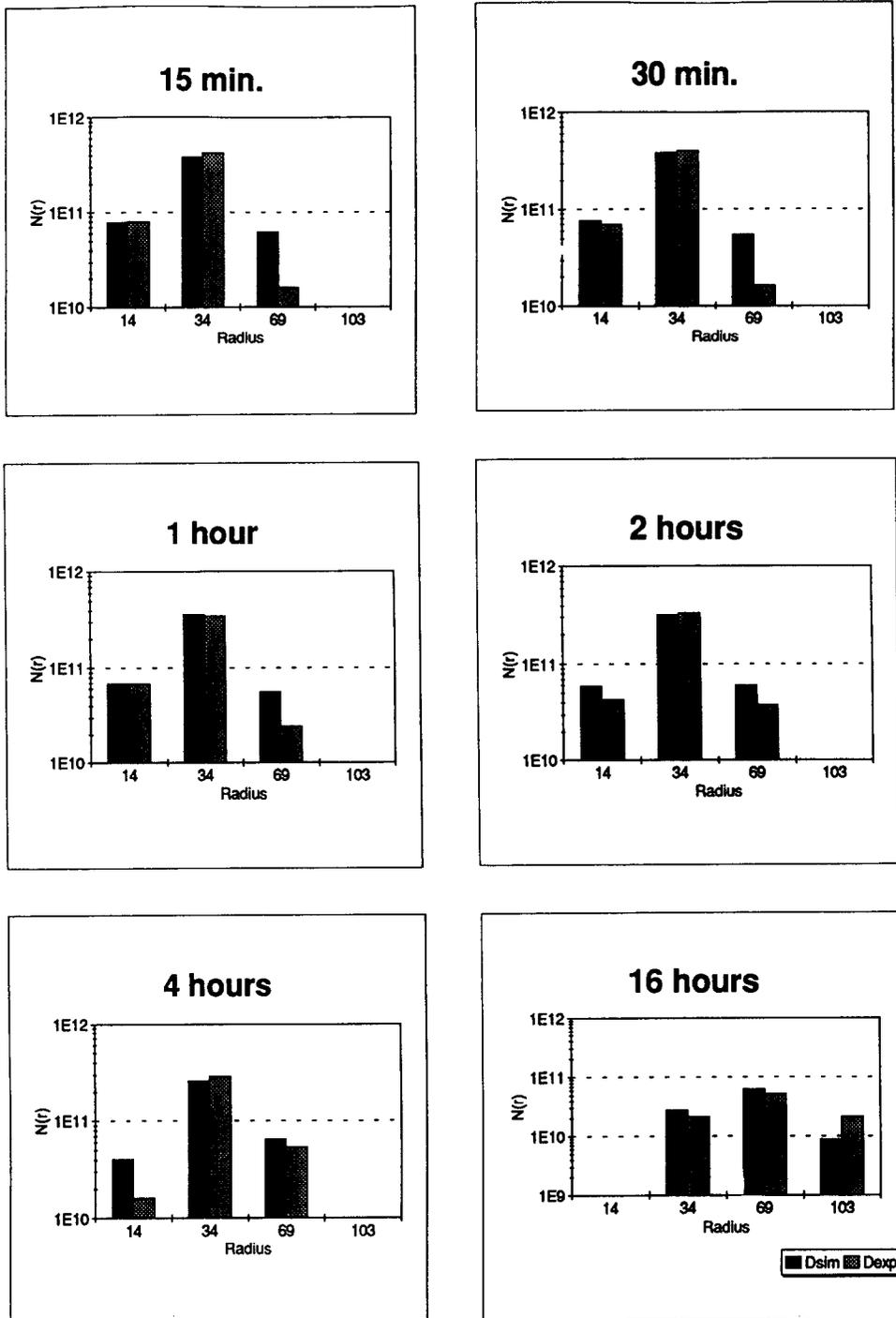
Fig. 1. Size spectra of loops as a function of loop radius after annealing in  $N_2$  at  $700^\circ C$  for annealing times ranging from 15 min to 16 h. The radius is in angstroms and the density is  $cm^{-2}$ .
