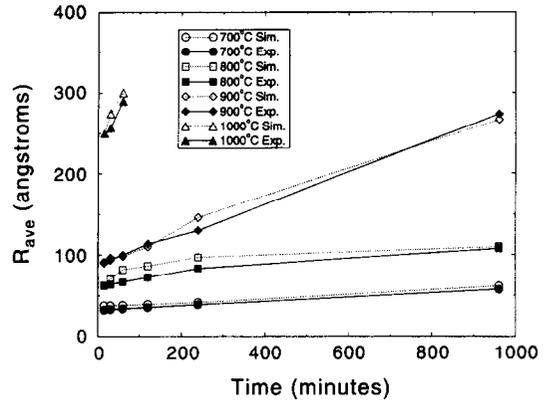
Fig. 5. Variation in average loop radius as a function of anneal time at different temperatures.
