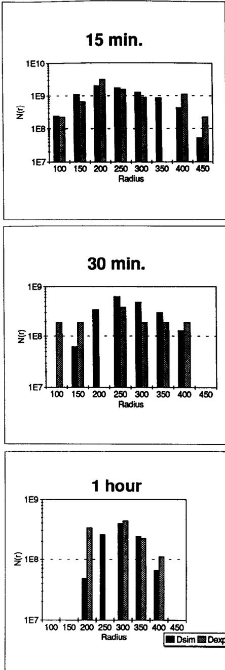
Fig. 4. Size spectra of loops as a function of loop radius after annealing in  $N_2$  at  $1000^\circ C$  for anneal times ranging from 15 min to 2 h. The radius is in angstroms and the density is  $cm^{-2}$ .
