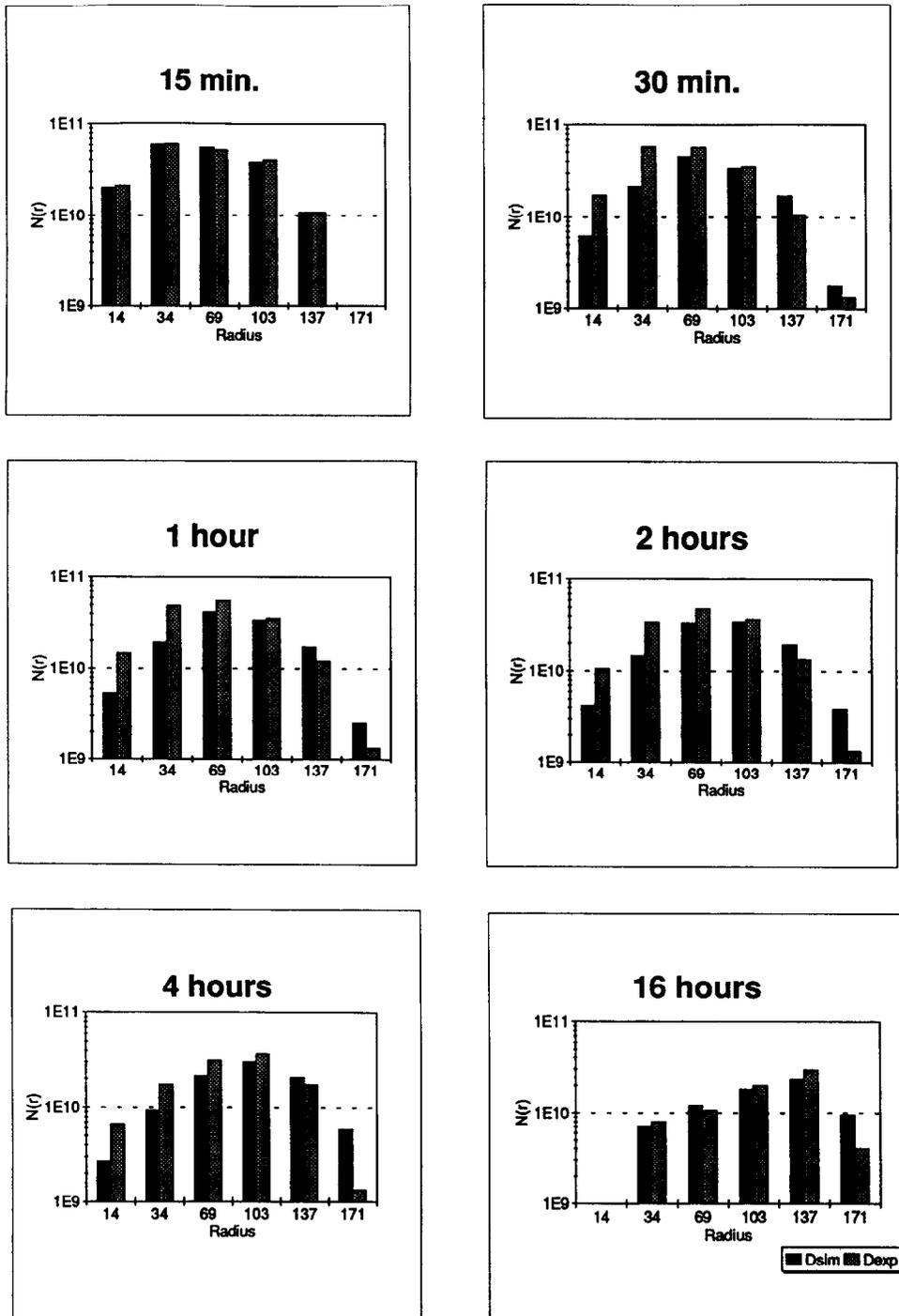
Fig. 2. Size spectra of loops as a function of loop radius after annealing in  $N_2$  at 800°C for anneal times ranging from 15 min to 16 h. The radius is in angstroms and the density is  $cm^{-2}$ .
