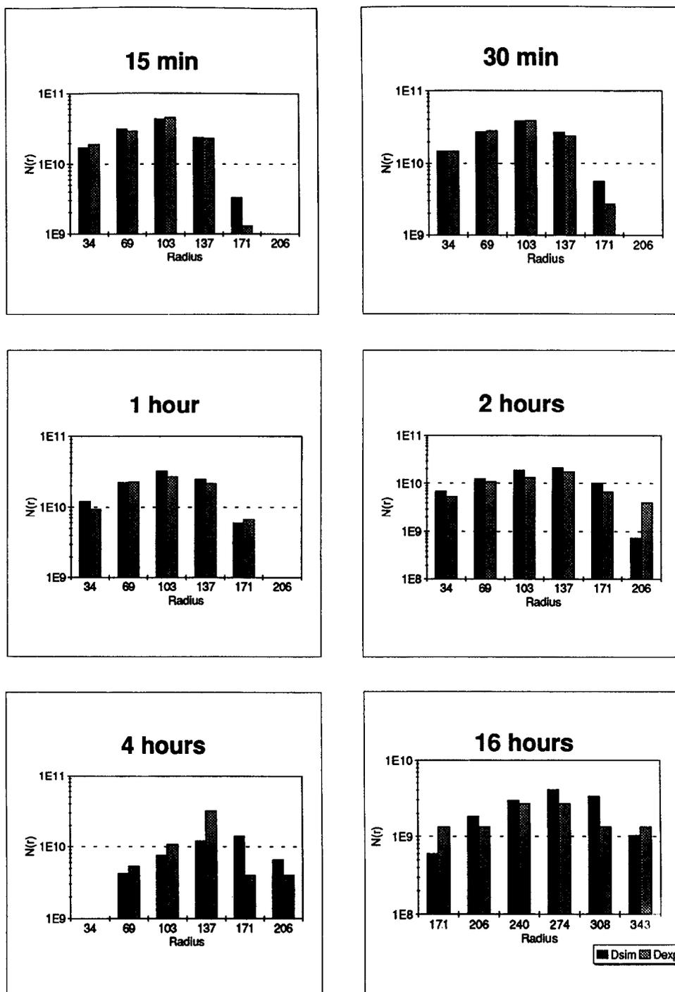
Fig. 3. Size spectra of loops as a function of loop radius after annealing in  $N_2$  at  $900^\circ\text{C}$  for anneal times ranging from 15 min to 16 h. The radius is in angstroms and the density is  $\text{cm}^{-2}$ .
