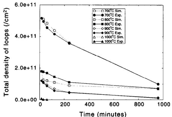
Fig. 6. Variation in total loop density as a function anneal time at different temperatures.
