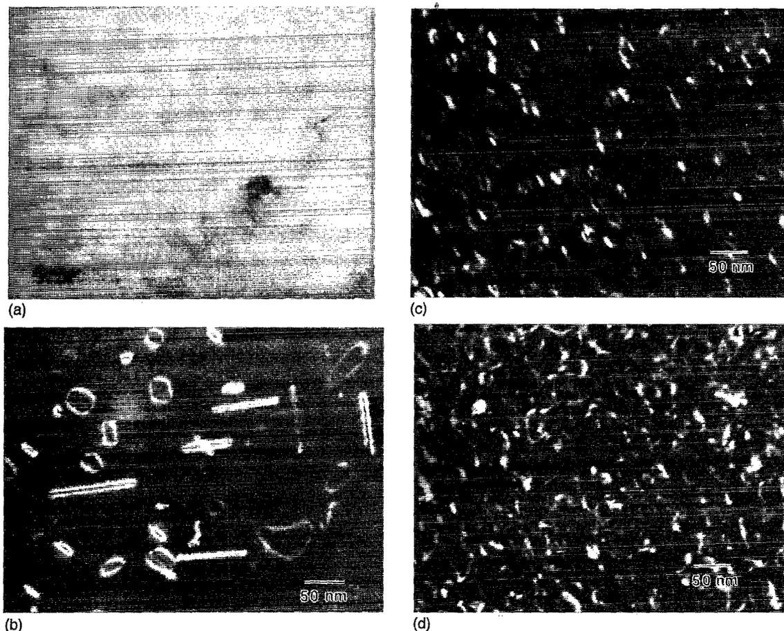
FIG. 1. Plan-view TEM micrographs of the samples annealed at 750 °C for 120 min for different doses, (a)  $4 \times 10^{15}/\text{cm}^2$ , bright field (BF), (b)  $8 \times 10^{15}/\text{cm}^2$ , weak-beam/dark-field (WBDF), (c)  $1.6 \times 10^{16}/\text{cm}^2$ , WBDF, (d)  $3.2 \times 10^{16}/\text{cm}^2$ , WBDF.
