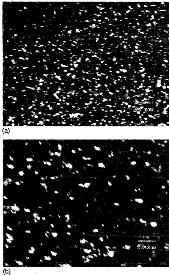
FIG. 2. Weak-beam/dark-field (WBDF) plan-view TEM micrographs of the samples implanted with 1.6×10<sup>16</sup> As/cm<sup>2</sup> and annealed at 700 °C for (a) 15 s, (b) 100 min.
