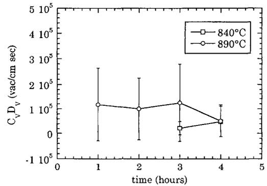
Fig. 5.  $C_V D_V$  values for the samples arrived at by solving Eq. (1) for various times, using the data from Fig. 4.
