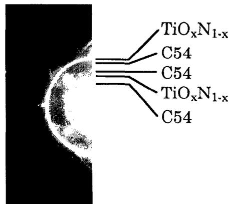
Fig. 2. Electron diffraction patterns of the films and Si substrate, showing the C54 TiSi<sub>2</sub> pattern and TiO<sub>x</sub>N<sub>1-x</sub> pattern. Note the double diffraction rings from the films.
