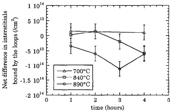
Fig. 4. Plot of the net difference in interstitials bound by the loops in the samples without a film and samples with a  $\text{TiSi}_2$  film.
