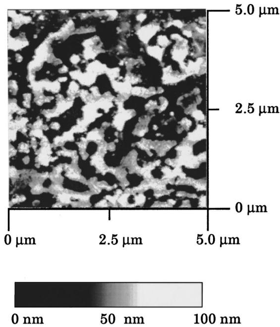
FIG. 1. Atomic force microscope micrograph of the underlying Si surface after chemical removal of the TiSi<sub>2</sub> film.
