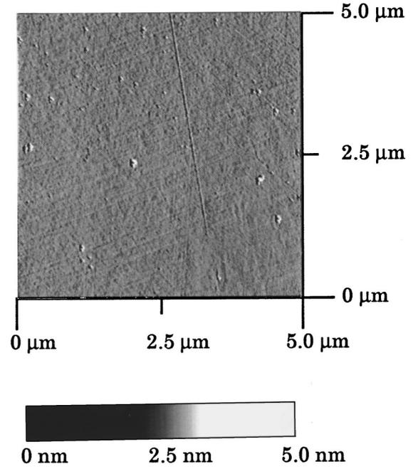
FIG. 3. Atomic force microscope micrograph of the underlying Si surface after chemical removal of the TiSi<sub>2</sub> film and chemo-mechanical polish.
