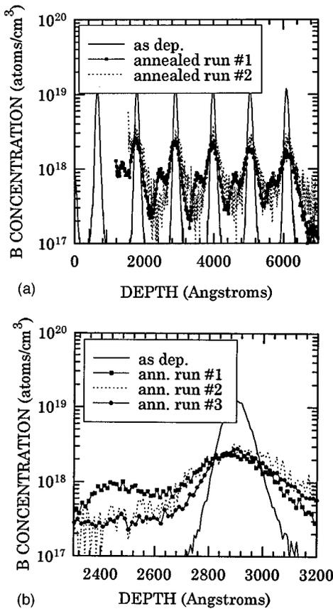
FIG. 2. (a) SIMS depth profiles of the silicided B doping superlattice after chemical removal of the TiSi<sub>2</sub> but without a chemo-mechanical polish of the surface. (b) Detailed graph of the third spike; three SIMS depth profiles were taken on different spots on the same sample.
