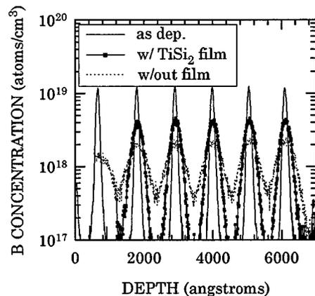
FIG. 4. SIMS depth profile of a silicided B doping superlattice annealed at 840 °C that has been CM polished after chemical removal of the TiSi<sub>2</sub> film.
