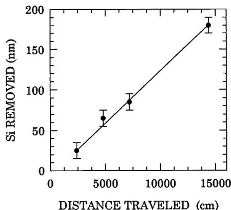
FIG. 6. Plot of the Si removed vs distance traveled on the polishing pad.
