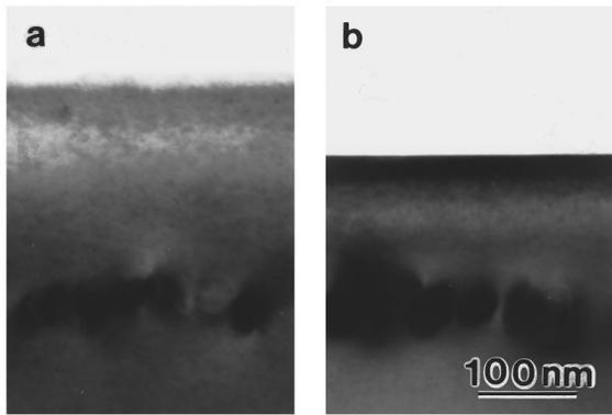
FIG. 5. XTEM micrographs of Si with a dislocation loop layer (a) before CMP polishing and (b) after 7300 cm travel on the pad during CMP.
