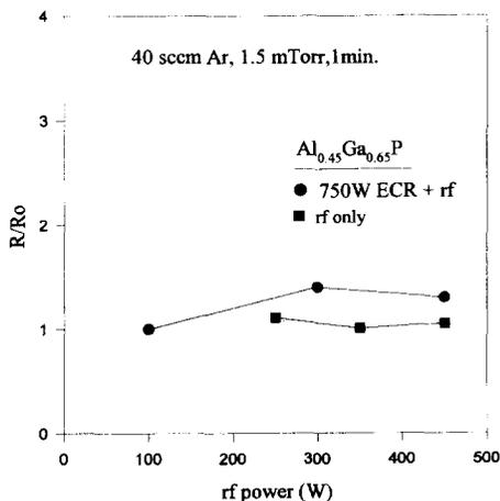
Fig. 1. Sheet resistance ratio increase in AlGaP after exposure to Ar plasmas, as a function of r.f. power.
