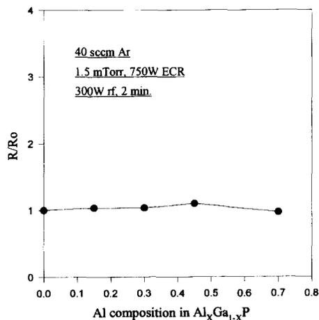
Fig. 2. Sheet resistance ratio increase in  $Al_xGa_{1-x}P$  as a function of Al composition.
