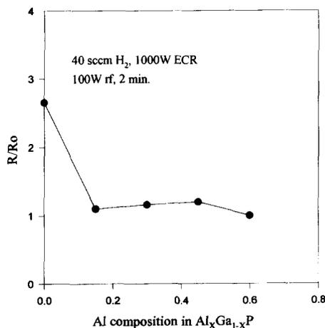
Fig. 5. Sheet resistance ratio increase in AlGaP after hydrogen plasma exposure, as a function of Al composition.
