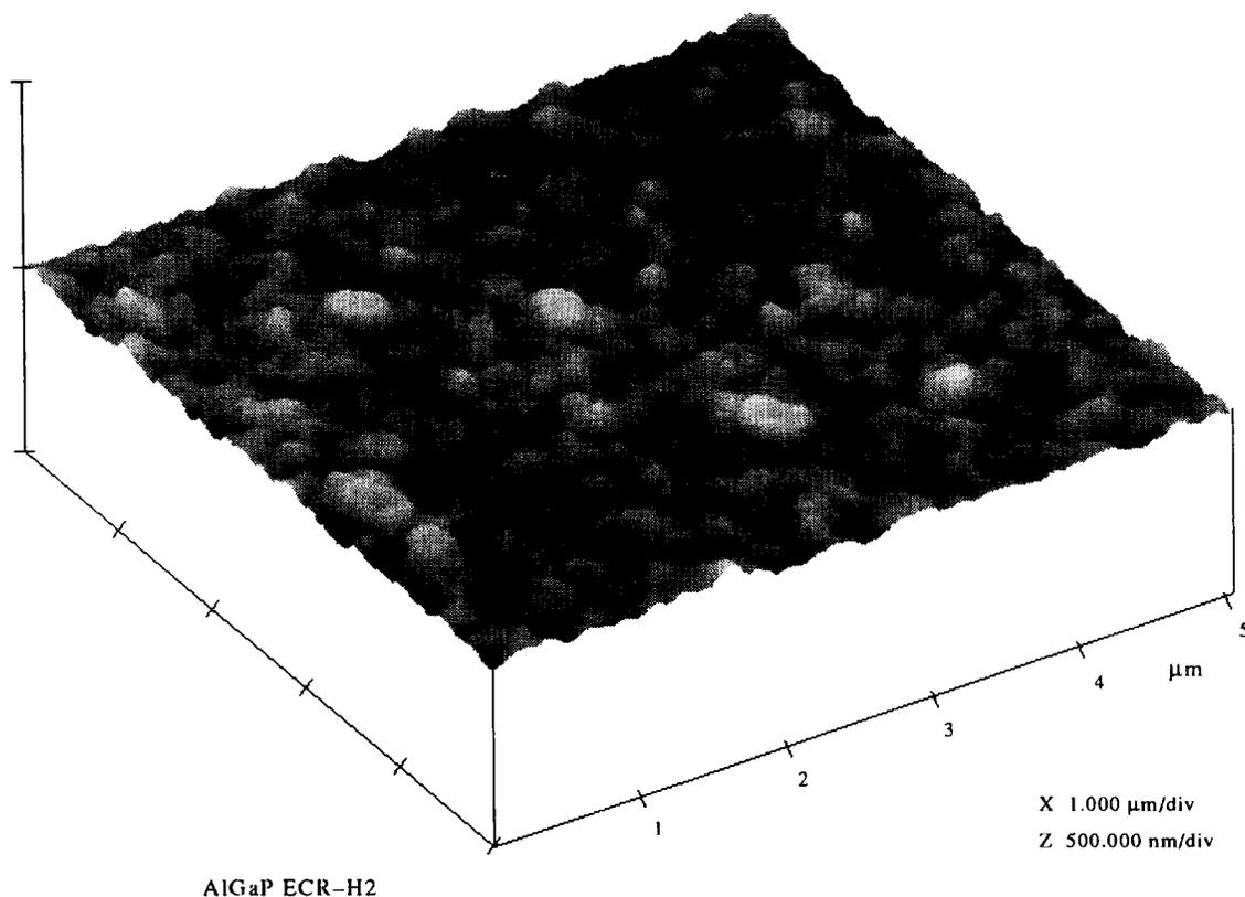
Fig. 7. AFM scan of H<sub>2</sub> plasma treated AlGaP.
