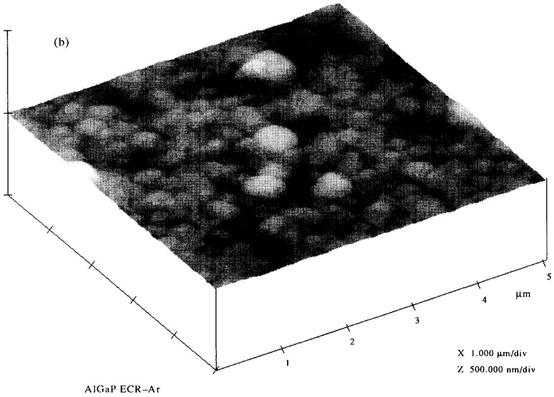
Fig. 4. (a) AFM scan as-grown AlGaP; (b) AFM scan of ECR Ar plasma-treated AlGaP.
