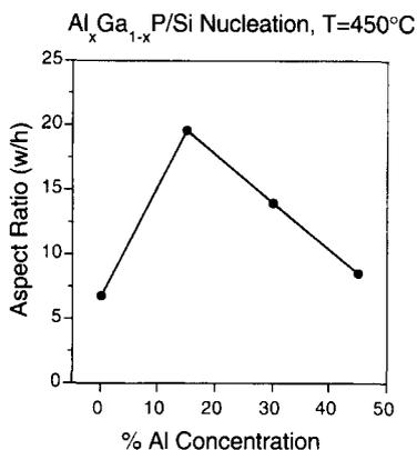
Fig. 4. Aspect ratio (width/height) of  $Al_xGa_{1-x}P$  islands deposited on silicon at 450°C.
