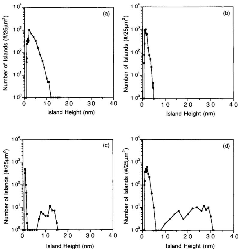
Fig. 5. Island size histograms for nucleation of  $Al_xGa_{1-x}P$  from  $25 \mu m^2$  scans (a) GaP/Si,  $T_G = 450^\circ C$ , (b)  $Al_{0.15}Ga_{0.85}P/Si$ ,  $T_G = 450^\circ C$ , (c)  $Al_{0.45}Ga_{0.55}P/Si$ ,  $T_G = 500^\circ C$ , and (d)  $Al_{0.45}Ga_{0.55}P/Si$ ,  $T_G = 550^\circ C$ .
