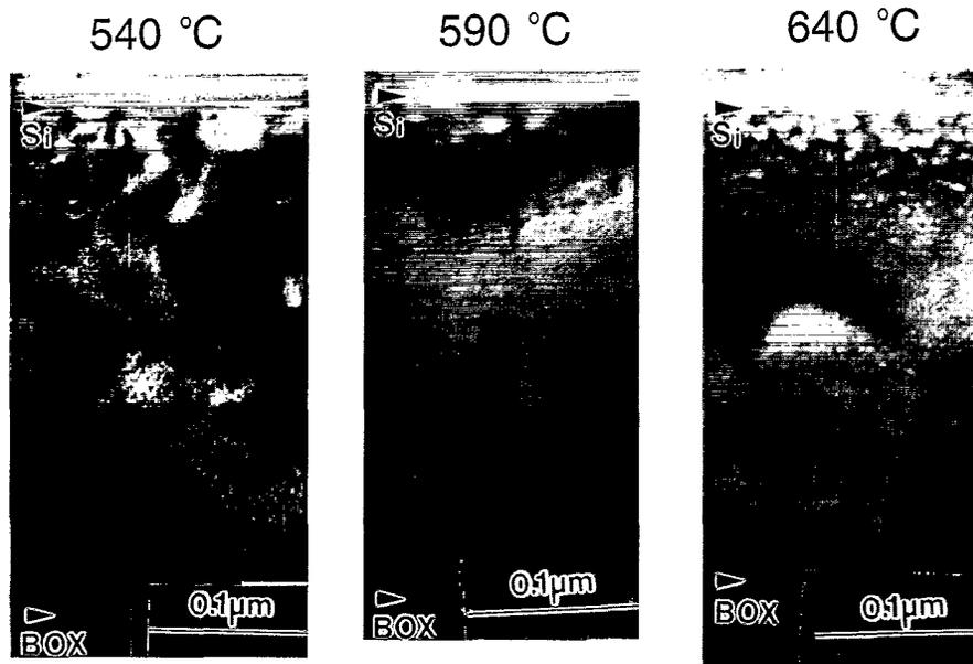
Fig. 1. TEM cross-sections of the Si layer for three different temperatures of implant.
