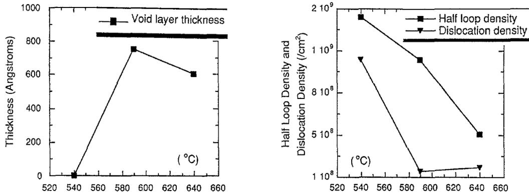
Fig. 2. Correlation of vacancy cluster formation depth at different substrate temperatures to ultimate threading dislocation density.
