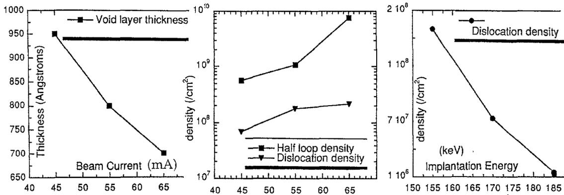
Fig. 4. Correlation of vacancy cluster formation. Dislocation depth at different beam currents (mA) with density for different ultimate threading dislocation density beam energies (keV).
