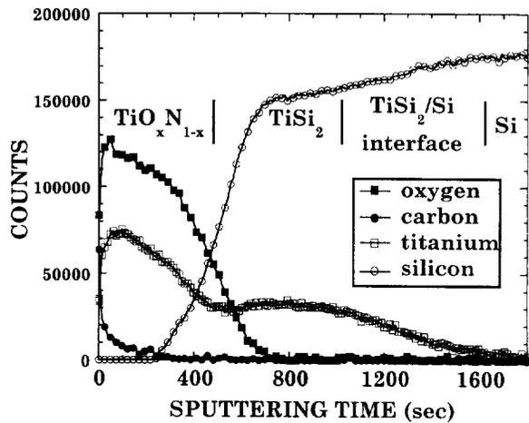
Fig. 2. Auger spectra from the annealed  $\text{TiSi}_{0.8}$  sample.
