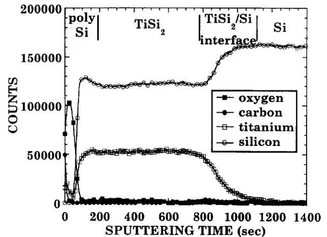
Fig. 3. Auger spectra from the annealed  $\text{TiSi}_{2.2}$  sample.
