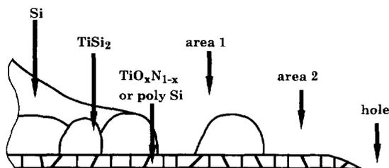
Fig. 8. Schematic cross-section of the PTEM samples.
