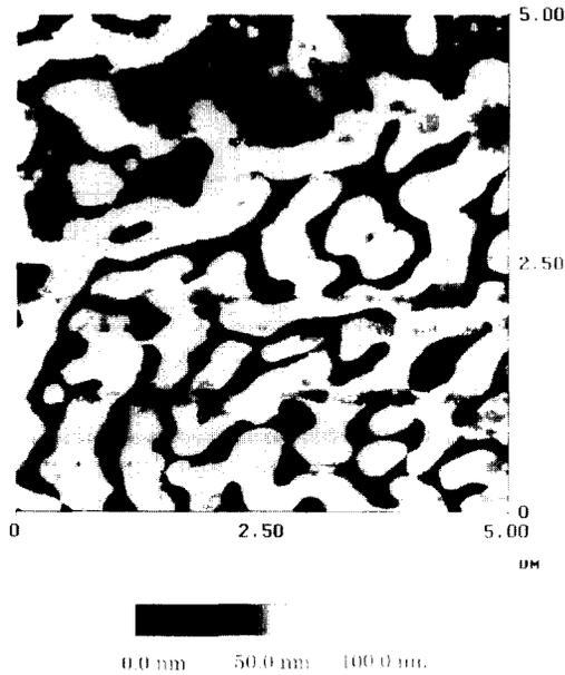
Fig. 5. Representative AFM micrograph of the underlying Si surface of Ti (only) sample after annealing and chemically etching off the films.
