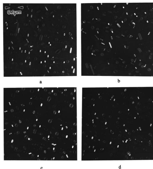
FIG. 3. Plan-view TEM of the evolution of the 70 keV  $\text{Si}^+$   $1 \times 10^{15}/\text{cm}^2$  EOR damage after (a) 1 keV  $\text{B}^+$  implant  $1 \times 10^{15}/\text{cm}^2$  and 1000 °C spike anneal (b) 5 keV  $\text{BF}_2^+$  implant  $1 \times 10^{15}/\text{cm}^2$  and 1000 °C spike anneal (c) 1 keV  $\text{B}^+$  implant  $1 \times 10^{15}/\text{cm}^2$  and 1050 °C spike anneal (d) 5 keV  $\text{BF}_2^+$  implant  $1 \times 10^{15}/\text{cm}^2$  and 1050 °C spike anneal.
