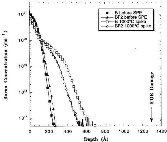
FIG. 1. Effect of F on B TED. SIMS of preamorphized silicon implanted with either 1 keV  $^{11}\text{B}$  or 5 keV  $\text{BF}_2$  profiles annealed at 550 °C for 30 s then at 1000 °C, 0 s in 33 ppm  $\text{O}_2+\text{N}_2$ .
