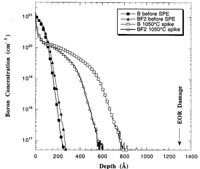
FIG. 2. Effect of F on B TED. SIMS of preamorphized silicon implanted with either 1 keV  $^{11}\text{B}$  or 5 keV  $\text{BF}_2$  profiles annealed at 550 °C for 30 s then 1050 °C, 0 s in 33 ppm  $\text{O}_2+\text{N}_2$ .
