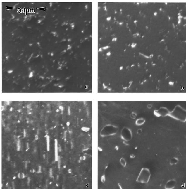
FIG. 2. Plan-view  $g_{220}$  TEM micrographs showing the effects of furnace annealing on implanted samples with (a) LTP processing after  $750^\circ\text{C}$  15 min annealing, (b) LTP processing after  $750^\circ\text{C}$  360 min annealing, (c) no LTP processing after  $750^\circ\text{C}$  15 min annealing, (d) no LTP processing after  $750^\circ\text{C}$  360 min annealing.
