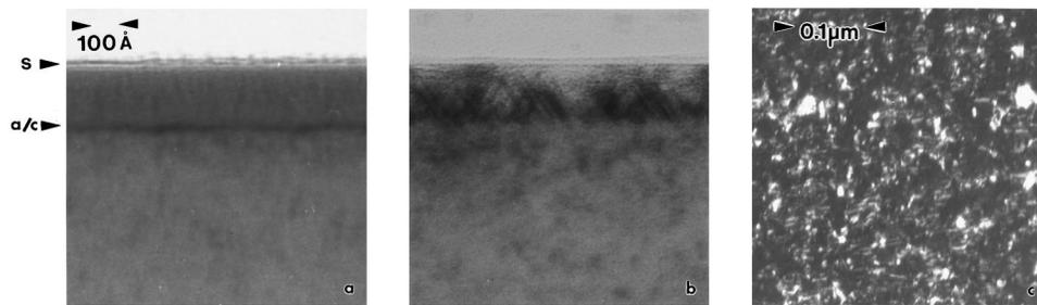
FIG. 1. Cross-sectional TEM micrographs for the (a) as-implanted sample,  $10 \text{ keV Si}^+ 1 \times 10^{15} \text{ cm}^{-2}$  (b) after laser thermal processing (c) plan-view TEM micrograph of the laser thermal processed sample. Note the high density of stacking faults and microtwins present after LTP processing.
