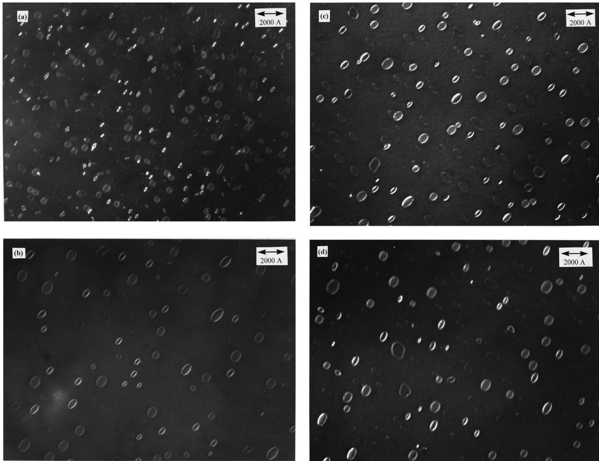
FIG. 1. TEM images of the samples of (a) the loop control and loop samples with loop depth of (b) 2600 Å, (c) 1800 Å, and (d) 1000 Å after the 1000 °C, 15 min anneal.
