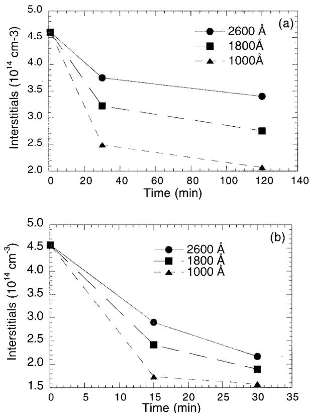
FIG. 3. Plot of loss of interstitials with time at (a) 900 °C and (b) 1000 °C for the three loop depths.
