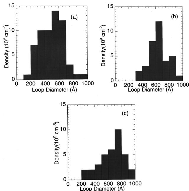
FIG. 2. Loop size distribution at 1000 °C, 30 min for (a) 2600 Å, (b) 1800 Å, and (c) 1000 Å loop depth samples.
