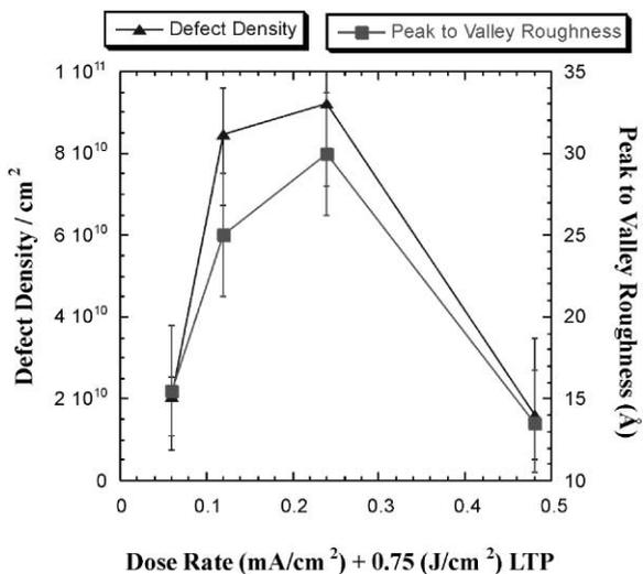
Fig. 4. Plot showing direct correlation between defect density and interfacial roughness.
