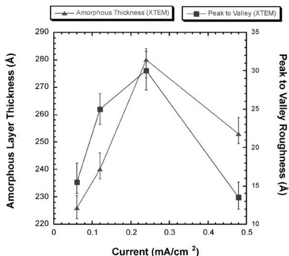
Fig. 1. Amorphous layer thickness and amorphous/crystalline interface roughness as a function of beam current for a 10 keV  $\text{Si}^+ 1 \times 10^{15} \text{ cm}^{-2}$  implant.
