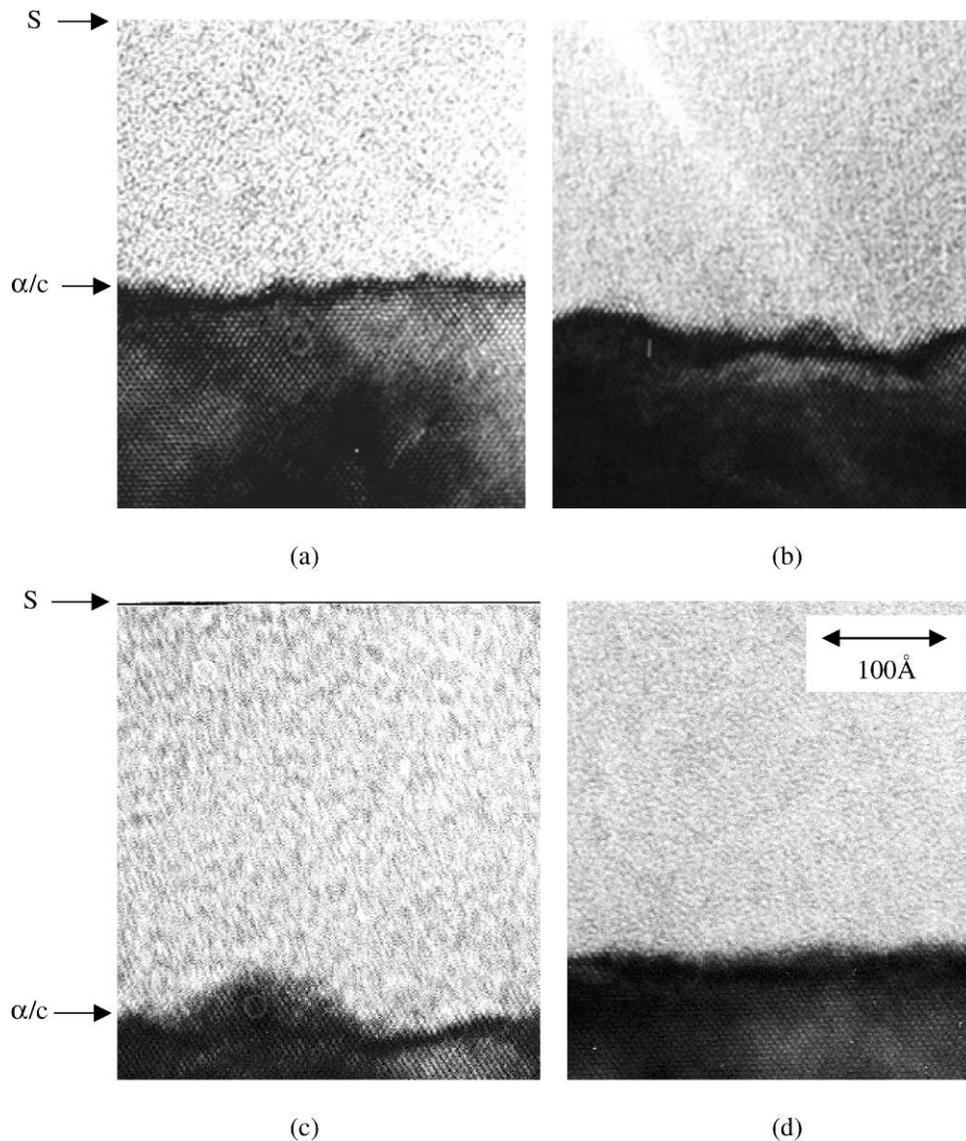
Fig. 2. HR-XTEM micrographs showing differences in amorphous layer thickness and a/c interfacial roughness for a 10 keV Si<sup>+</sup>  $1 \times 10^{15}$  cm<sup>-2</sup> implant at different beam currents. (a) 0.06 mA with a-depth of 226 Å, (b) 0.12 mA with a-depth of 240 Å, (c) 0.24 mA with a-depth of 280 Å, and (d) 0.48 mA with a-depth of 253 Å.
