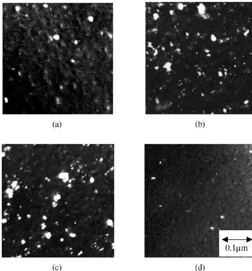
Fig. 3. Plan-view  $g_{220}$  TEM micrographs of different beam currents plus  $0.75 \text{ J/cm}^2$  LTP. (a)  $0.06 \text{ mA}$ , (b)  $0.12 \text{ mA}$ , (c)  $0.24 \text{ mA}$ , (d)  $0.48 \text{ mA}$ . Decrease in number of defects in (a) and (d), corresponding to a reduction in a/c interfacial roughness.
