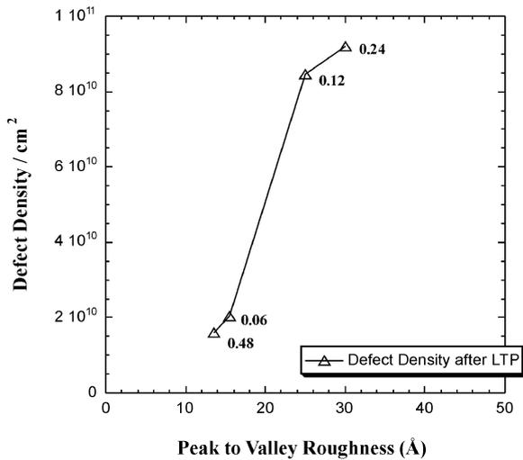
Fig. 5. A dose rate of 0.48 mA/cm<sup>2</sup> significantly reduces a/c interfacial roughness and therefore, defect density.
