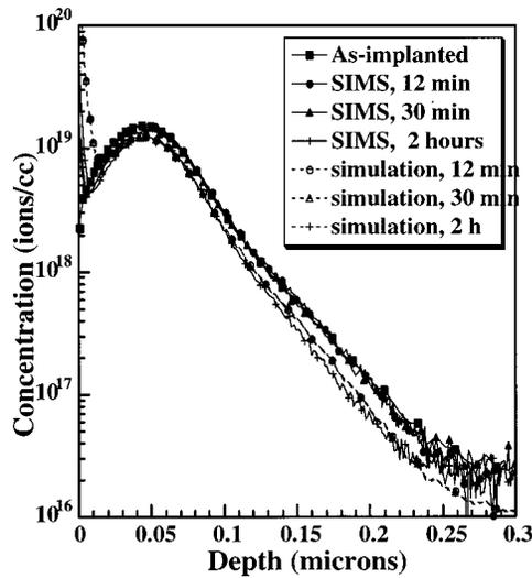
FIG. 2. SIMS vs simulations comparisons at 650 °C for  $5 \times 10^{13} \text{ N}_2^+$ , 40 keV.
