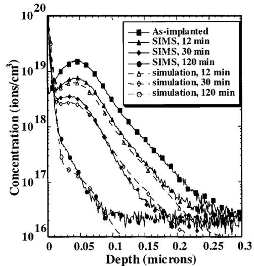
FIG. 1. SIMS vs simulations comparisons at 750 °C for  $5 \times 10^{13} N_2^+$ , 40 keV.
