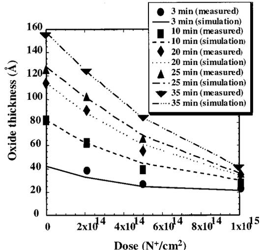
FIG. 6. Oxide thickness vs implanted nitrogen dose at different oxidation times at 900 °C. The oxide thickness data are as published in Ref. 14.
