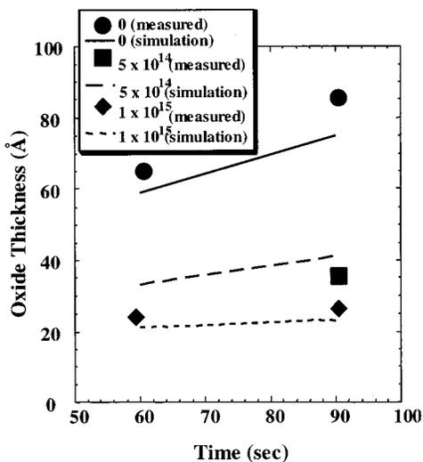
FIG. 8. Oxide thickness vs RTO time for different implanted nitrogen doses at 1050 °C. The oxide thickness data is as in Ref. 14.
