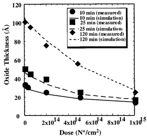
FIG. 7. Oxide thickness vs implanted nitrogen dose at different times at 800 °C. The oxide thickness data are as published in Ref. 14.
