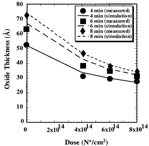
FIG. 5. Oxide thickness vs implanted nitrogen dose at different times at 900 °C.
