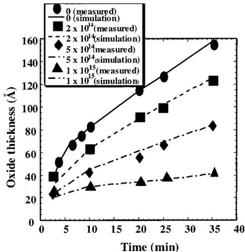
FIG. 4. Plot of oxide thickness vs time at 900 °C for  $I/I N^+$  doses. We measured some of the data and the rest were obtained from Ref. 14.
