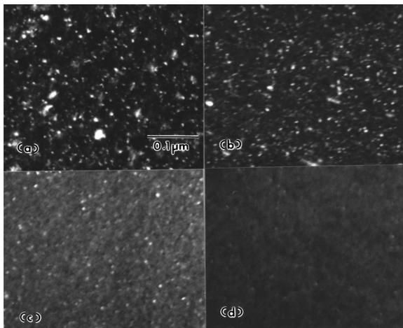
FIG. 4. WDF  $g_{220}$  plan-view transmission electron micrographs of the damage created by a SIMS depth profile after annealing at 750 °C for 30 min, at distances of (a) 0.6–0.8, (b) 1.0–1.2, (c) 1.4–1.6, and (d) 1.8–2.0 mm from the original SIMS crater.
