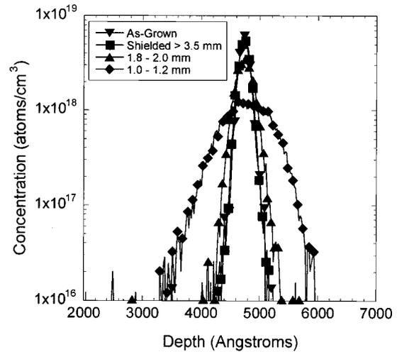
FIG. 2. SIMS depth profiles of the boron marker layer after annealing at 750 °C for 30 min, as a function of distance from the original SIMS crater.
