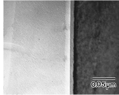
FIG. 5. Bright-Field XTEM micrograph of the amorphous layer created by SIMS depth profiling. The amorphous layer is 78 Å thick and is shown as the light-gray region bordering the rough dark band.
