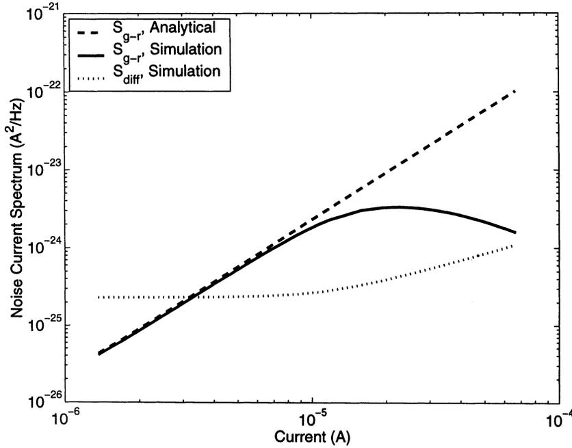
Fig. 2. Comparison between the simulated and analytical g-r current noise spectral density as a function of the bias voltage ( $f = 1$  Hz). The dashed line represents expression (9). The solid line is the simulated g-r noise. The dotted line is the simulated velocity fluctuation noise.
