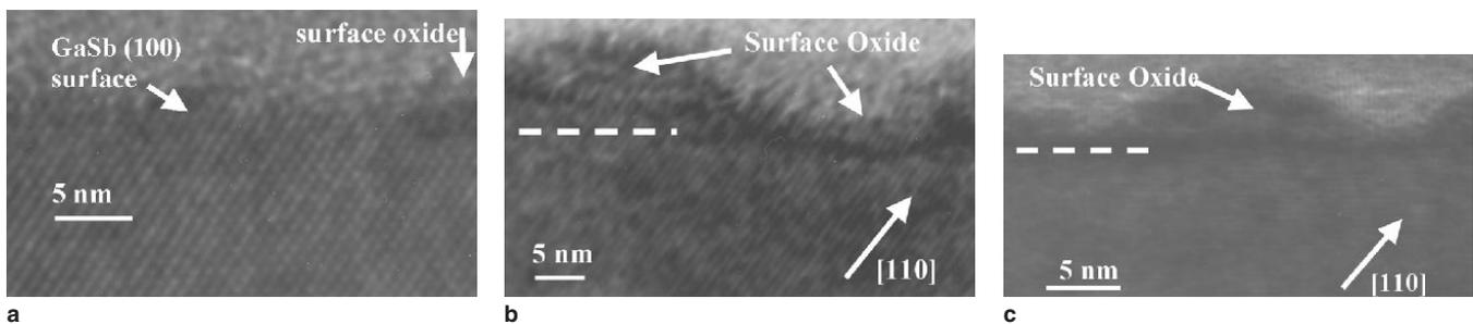
Fig. 4. (a) The HRTEM cross-section image of the pre-GCIB (as-received) GaSb(100). (b) The HRTEM cross-section image of the post-GCIB (dual-energy [10-kV, 3-kV]  $\text{CF}_4/\text{O}_2$ ) process. (c) The HRTEM cross-section image of the dual-energy [10-kV, 3-kV], dual-gas-species process with oxygen GCIB as the final step.
