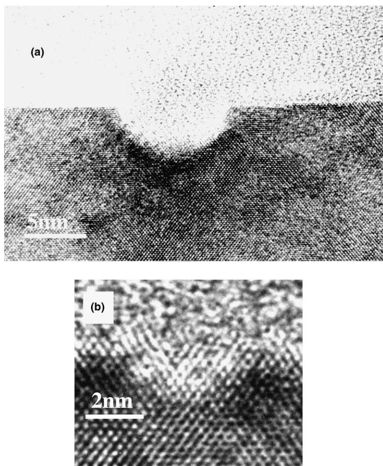
Fig. 5. (a) HRTEM cross-section image of an individual 24 kV  $O_2$  gas cluster ion impact into Si(1 1 1). Rounder impact craters typically resulted from the  $O_2$  cluster process, perhaps from the immediate oxidation of the Si and the change in associated bond strength of the forming crater wall; (b) HRTEM cross-section of an individual 3 kV  $O_2$  gas cluster impact into Si(1 1 1). The rounder shape of the impact is preserved with the shallow depth of the crater.
