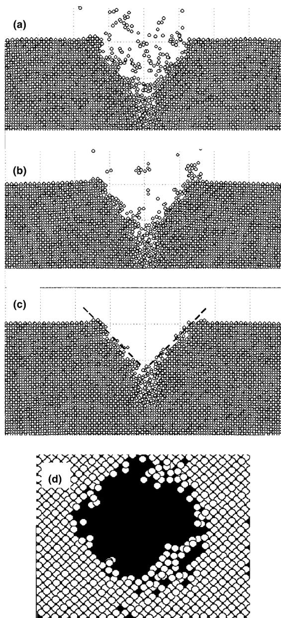
Fig. 1. (a) MD result for the three time instants for side-views of the crater formed by a 25 eV/atom  $\text{Ar}_{369}$  cluster impact on a  $\text{Si}(1\ 0\ 0)$  surface after time intervals: (a) 2.9, (b) 5.8 and (c) 14.4 ps from the start of cluster collision with the target; d) top-view of the crater formed by a  $\text{Ar}_{135}$ , 25 eV/atom, cluster impact on a  $\text{Si}(1\ 0\ 0)$  surface.
