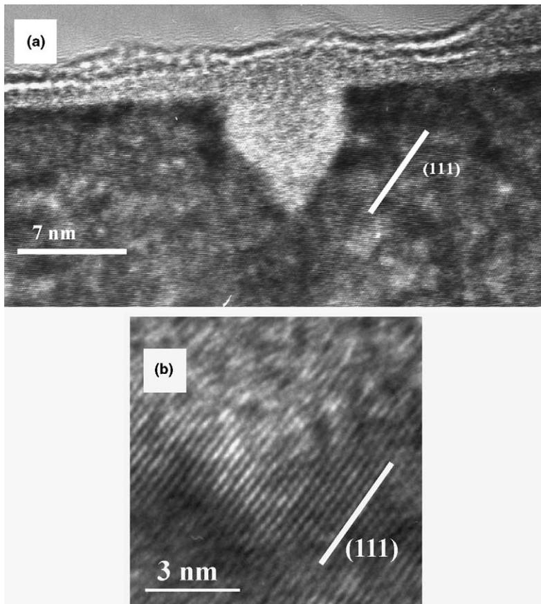
Fig. 4. (a) HRTEM cross-section image of an individual 24 kV Ar gas cluster ion impact into Si(100). Crater conical edges align along the (111) lattice planes; (b) HRTEM cross-section image of an individual 3 kV Ar gas cluster ion impact into Si(100). Crater conical edges align along the (111) lattice planes, but the depth of impact is reduced.
