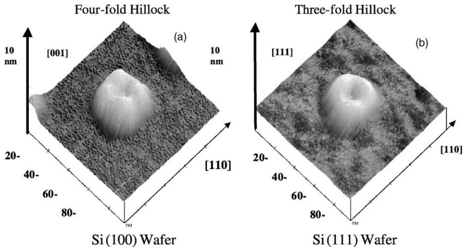
Fig. 6. Three-dimensional AFM image of four fold symmetry of Si(100) 24 kV Ar cluster impact hillock (a) and three fold symmetry of Si(111) 24 kV Ar cluster impact hillock (b). Dimensions of both AFM images are 100 nm  $\times$  100 nm with a 10 nm height scaling.
