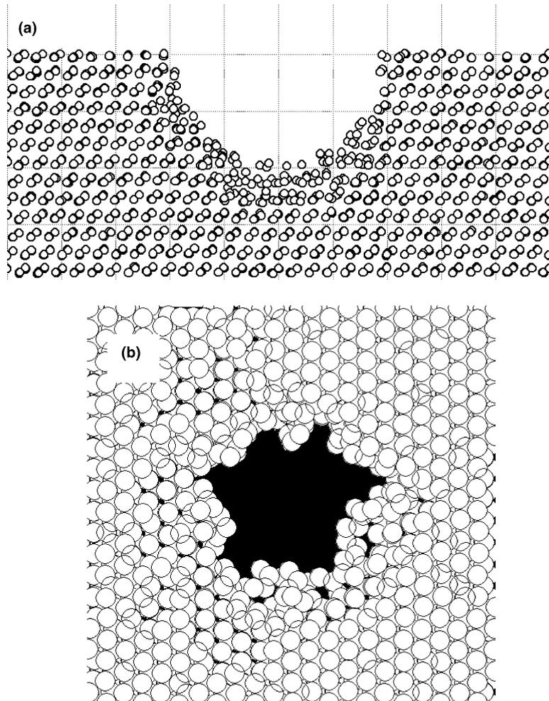
Fig. 2. (a) MD result for the side-view of a crater formed on a Si(111) surface by a  $\text{Ar}_{135}$  cluster impact, with energy of 25 eV/atom, 14.4 ps after the beginning of impact. (b) Top-view of the crater formed on a Si(111) surface by an  $\text{Ar}_{135}$ , 25 eV/atom, cluster impact. The complicated faceting feature is clearly seen and may be compared with the AFM image of Fig. 4.
