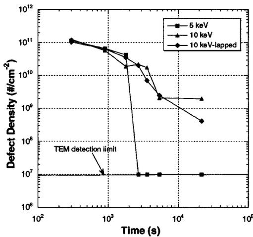
FIG. 4. Defect density evolution of the 10 keV-lapped samples annealed at 750 °C compared to the 10 and 5 keV energies. The 10 keV-lapper specimen follows the same trend as the 10 keV energy. This shows that EOR surface proximity is not the factor for the 5 keV defect dissolution.
