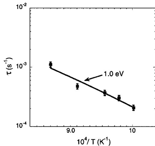
FIG. 6. Activation energy plot showing the defect dissolution times and temperatures. A best-fit exponential curve results in activation energy of 1.0±0.1 eV.
