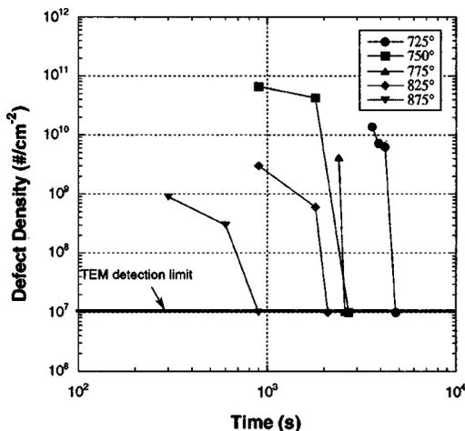
FIG. 5. Defect density over time for five temperatures near their dissolution times for the 5 keV energy at 750 °C. The dissolution process occurs rapidly, there is not a gradual decrease in defects over time as in higher energies.
