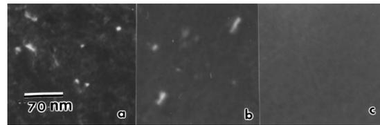
FIG. 3. Plan-view TEM micrographs for 60 min annealing times at 750 °C for (a) 10 keV, (b) 10 keV-lapped, and (c) 5 keV samples. Note that the 10 keV-lapped specimen follows the same defect evolution as the normal 10 keV energy.
