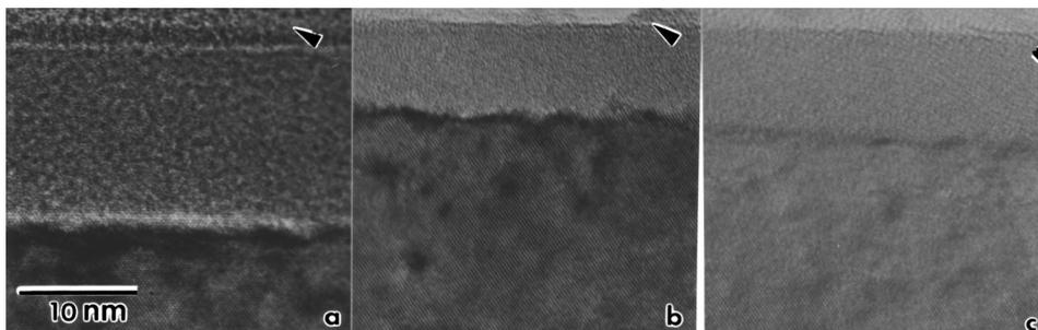
FIG. 2. High-resolution cross section NTEM micrographs of the amorphous layer thickness for (a) 10 keV, (b) 10 keV-lapped, and (c) 5 keV samples. 10 keV implants form an amorphous layer 180 Å thick. Arrows point to the surface layer. The 10 keV-lapped specimen's amorphous layer was reduced to 80 Å, less than the 100 Å 5 keV amorphous layer thickness.
