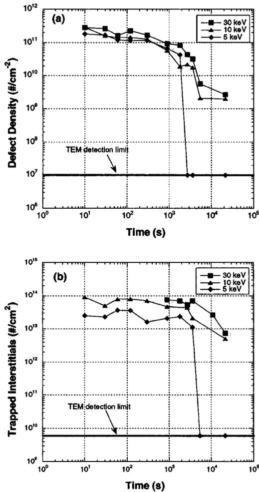
FIG. 1. Defect evolution of 30, 10, and 5 keV  $\text{Ge}^+$  implants at 750 °C. After 45 min of annealing, complete defect dissolution occurs at the 5 keV energy as shown by (a) defect density and (b) trapped interstitials over time. The two higher energies form stable dislocation loops that are stable after 360 min anneals.
