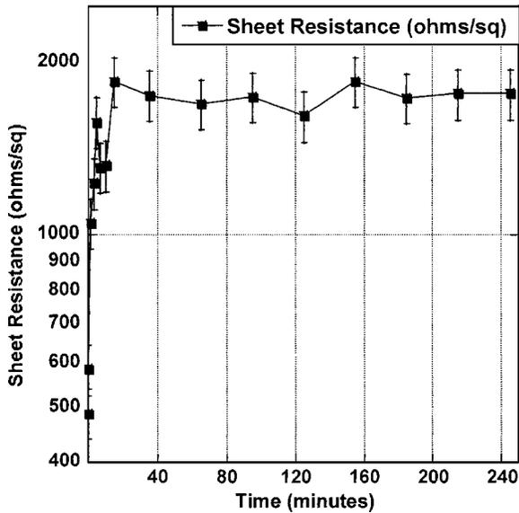
FIG. 7. Sheet resistance vs anneal time for samples containing a 1 keV,  $1 \times 10^{15} \text{ cm}^{-2} \text{ B}^+$  and 10 keV,  $1 \times 10^{15} \text{ cm}^{-2} \text{ Ge}^+$  implants. Annealed at 750 °C.
