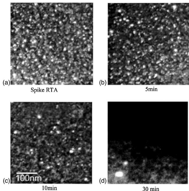
FIG. 2. PTEM WBDF images taken at  $g_{220}$  imaging conditions of the extended defects for samples containing  $1 \text{ keV}, 1 \times 10^{15} \text{ cm}^{-2} \text{ B}^+$  and  $10 \text{ keV}, 1 \times 10^{15} \text{ cm}^{-2} \text{ Ge}^+$  implants. Annealed at  $750 \text{ }^\circ\text{C}$ .
