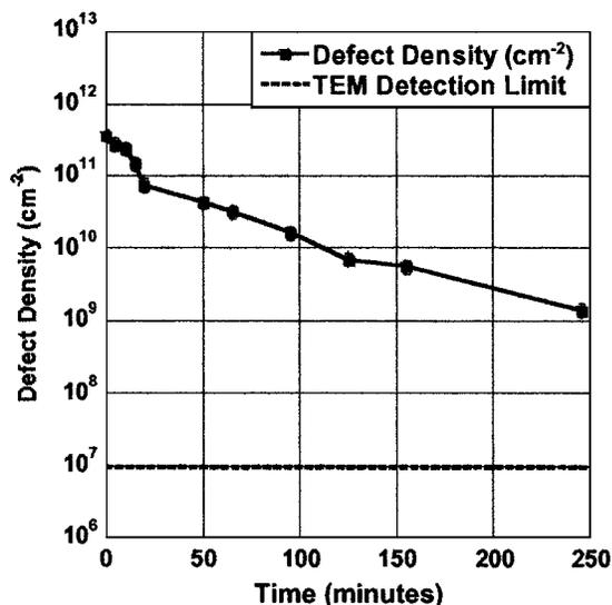
FIG. 5. Defect density as a function of annealing time for samples containing 10 keV,  $1 \times 10^{15} \text{ cm}^{-2}$  Ge<sup>+</sup> implants. Annealed at 750 °C.
