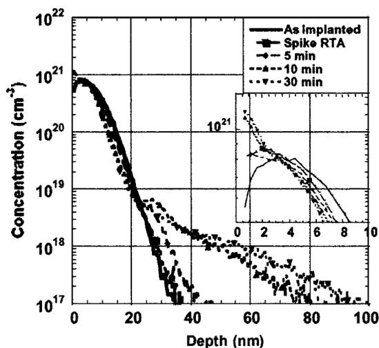
FIG. 6. Boron concentration-depth profiles for samples containing a 1 keV,  $1 \times 10^{15} \text{ cm}^{-2}$  B<sup>+</sup> and 10 keV,  $1 \times 10^{15} \text{ cm}^{-2}$  Ge<sup>+</sup> implants. Annealed at 750 °C.
