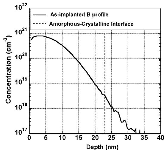
FIG. 1. As-implanted boron concentration-depth profile for sample containing a 1 keV,  $1 \times 10^{15} \text{ cm}^{-2}$  B<sup>+</sup> and 10 keV,  $1 \times 10^{15} \text{ cm}^{-2}$  Ge<sup>+</sup> implants, indicating the amorphous-crystalline interface.
