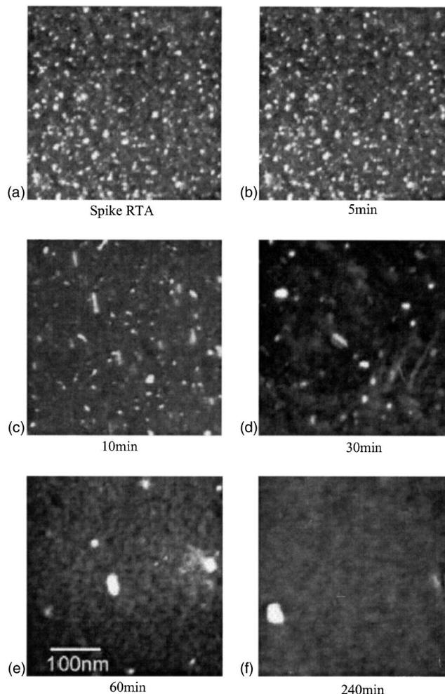
FIG. 4. PTEM WBDF images taken at  $g_{220}$  imaging conditions of the extended defects for samples containing  $10 \text{ keV}, 1 \times 10^{15} \text{ cm}^{-2} \text{ Ge}^+$  implants. Annealed at  $750 \text{ }^\circ\text{C}$ .
