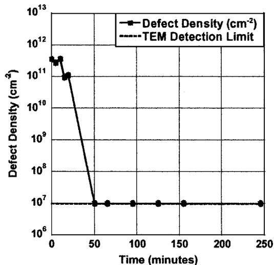
FIG. 3. Defect density as a function of annealing time for samples containing  $1 \text{ keV}, 1 \times 10^{15} \text{ cm}^{-2} \text{ B}^+$  and  $10 \text{ keV}, 1 \times 10^{15} \text{ cm}^{-2} \text{ Ge}^+$  implants. Annealed at  $750 \text{ }^\circ\text{C}$ .
