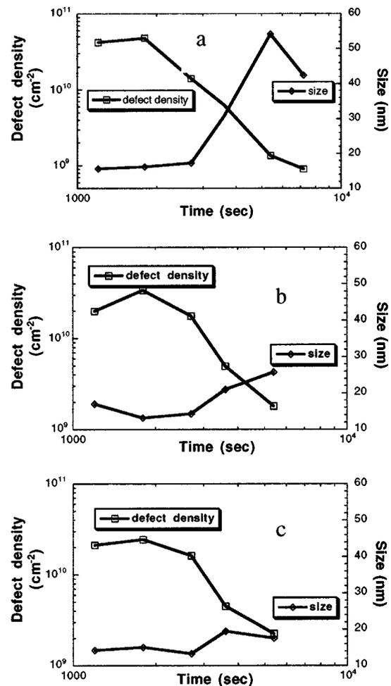
FIG. 2. {311} defect density and size of the low Ge regime alloys, (a) pure Si, (b)  $\text{Si}_{0.98}\text{Ge}_{0.02}$ , and (c)  $\text{Si}_{0.95}\text{Ge}_{0.05}$ , annealed at  $750 \text{ }^\circ\text{C}$ .
