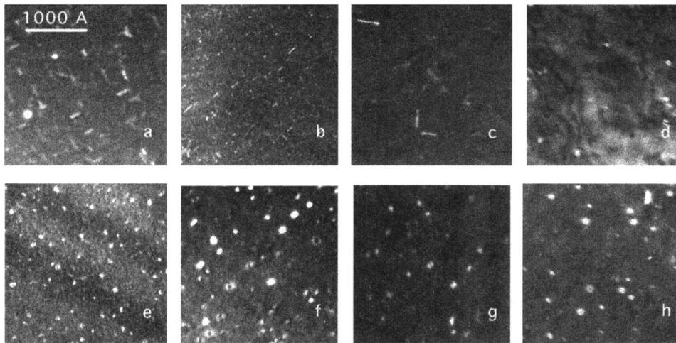
FIG. 1. PTEM images of 40 keV,  $1 \times 10^{14} \text{ cm}^{-2}$  Si implant into relaxed  $\text{Si}_{0.98}\text{Ge}_{0.02}$  [(a) 30 min, (b) 45 min, (c) 60 min, and (d) 120 min] and  $\text{Si}_{0.75}\text{Ge}_{0.25}$  [(e) 30 min, (f) 45 min, (g) 60 min, and (h) 120 min] annealed at  $750 \text{ }^\circ\text{C}$ .
