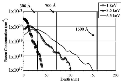
FIG. 1. UT-MARLOWE ion profile simulations for  $\text{B}^+$  implants at 1 keV, 3.5 keV, 6.5 keV,  $3 \times 10^{14} \text{ cm}^{-2}$ . Note location of surface Si/BOX interface for 300 Å, 700 Å, and 1600 Å SOI.
