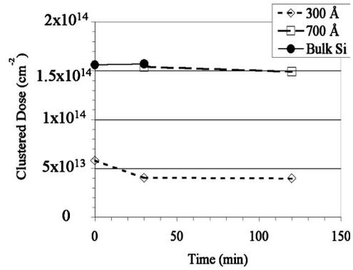
FIG. 9. Clustered dose in SOI and bulk Si for B<sup>+</sup>, 6.5 keV, 3 × 10<sup>14</sup> cm<sup>-2</sup> annealed at 750 °C. Dose was obtained by integrating the B concentration profiles that lie above a level of 1 × 10<sup>19</sup> cm<sup>-3</sup>.
