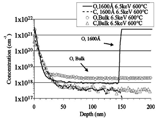
FIG. 11. Carbon and oxygen SIMS profiles for 1600 Å SOI and bulk Si implanted with B<sup>+</sup>, 6.5 keV,  $3 \times 10^{14} \text{ cm}^{-2}$ , and annealed at 600 °C for 30 min.
