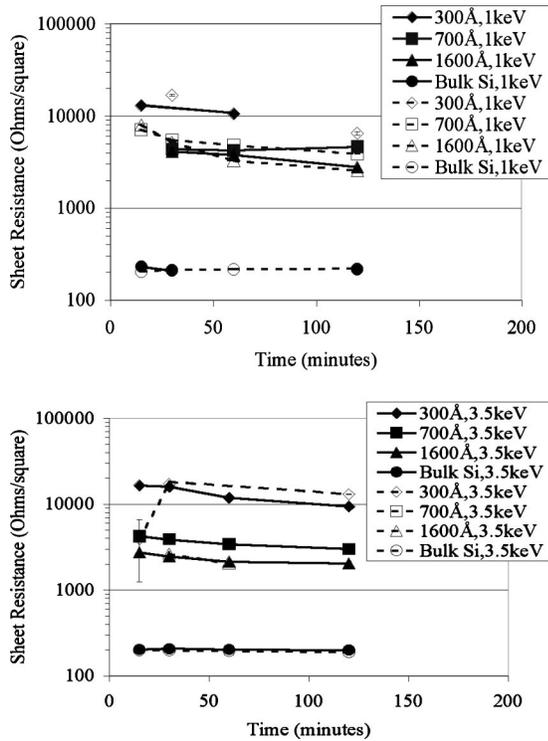
FIG. 5. Comparison of sheet resistance data measured by four-point probe and Hall effect for (a) 1 keV, (b) 3.5 keV, and (c) 6.5 keV,  $3 \times 10^{14} \text{ cm}^{-2}$  annealed at 750 °C. Solid symbols and lines represent four-point probe measurements and open symbols represent Hall measurements.
