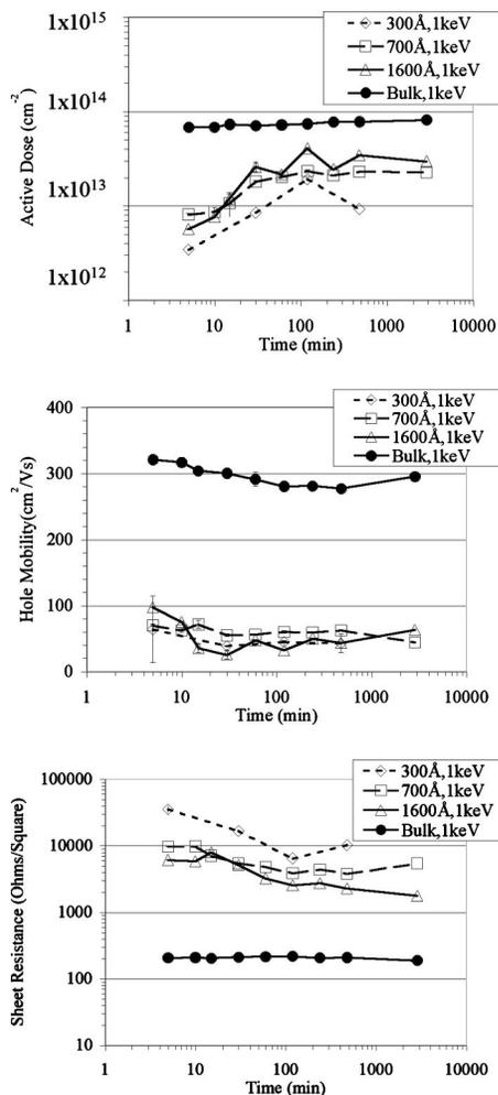
FIG. 3. Isothermal Hall data for B<sup>+</sup>, 1 keV,  $3 \times 10^{14}$  cm<sup>-2</sup> at 750 °C including (a) active dose, (b) hole mobility, and (c) sheet resistance.
