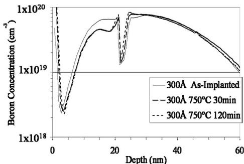
FIG. 8. Boron concentration profiles from SIMS for 300 Å SOI implanted at 6.5 keV, 3 × 10<sup>14</sup> cm<sup>-2</sup> then annealed at 750 °C. Note segregation of boron into buried oxide.
