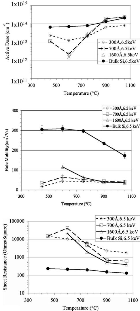
FIG. 7. Isochronal Hall data for B<sup>+</sup>, 6.5 keV, 3 × 10<sup>14</sup> cm<sup>-2</sup> after annealing for 30 min showing (a) active dose, (b) hole mobility, and (c) sheet resistance.
