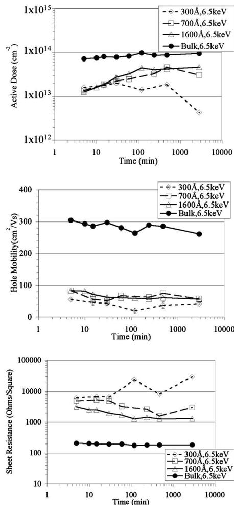
FIG. 4. Isothermal Hall data for B<sup>+</sup>, 6.5 keV,  $3 \times 10^{14}$  cm<sup>-2</sup> at 750 °C including (a) active dose, (b) hole mobility, and (c) sheet resistance.
