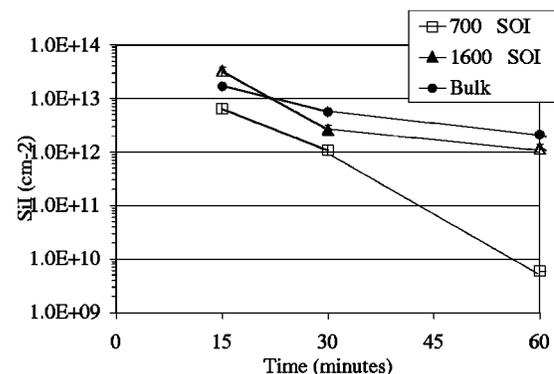
FIG. 2. Trapped interstitial concentration (Si<sub>i</sub>) as a function of annealing time for B<sup>+</sup>, 6.5 keV,  $3 \times 10^{14} \text{ cm}^{-2}$  specimens.
