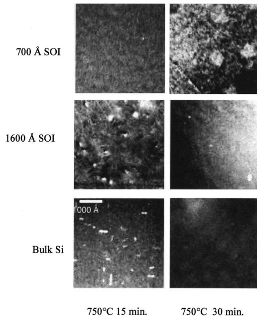
FIG. 1. PTEM WBDF micrographs of defect evolution in SOI and bulk for B<sup>+</sup>, 6.5 keV,  $3 \times 10^{14} \text{ cm}^{-2}$ .
