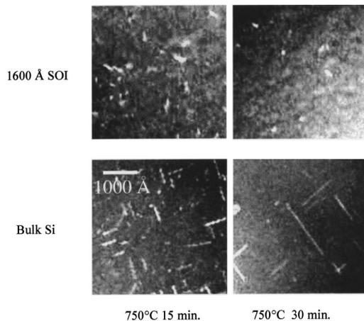
Fig. 4. PTEM WBDF micrographs of defect evolution in SOI and bulk for  $B^+$ , 19 keV,  $3 \times 10^{14} \text{ cm}^{-2}$ .
