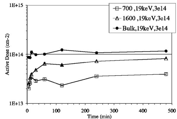
Fig. 6. Active dose of boron with annealing time for  $B^+$ , 19 keV,  $3 \times 10^{14} \text{ cm}^{-2}$  specimens measured using Hall effect. Error bars are smaller than the symbol size.
