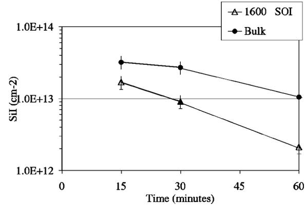
Fig. 5. Concentration of trapped interstitials as a function of time for  $B^+$ , 19 keV,  $3 \times 10^{14} \text{ cm}^{-2}$  specimens.
