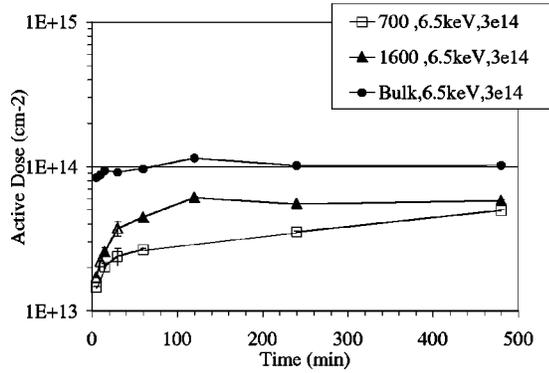
Fig. 3. Active dose of boron with annealing time for  $B^+$ , 6.5 keV,  $3 \times 10^{14} \text{ cm}^{-2}$  specimens measured using Hall effect.
