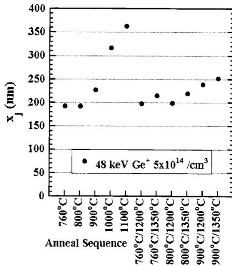
FIG. 5. Graph of  $x_j$  as a function of the anneal sequence for the 48-keV  $\text{Ge}^+$  preamorphization implant to  $5 \times 10^{14} \text{ cm}^{-2}$ . Note that all the samples that received either a 1200 or a 1350 °C fRTP anneal have shallower  $x_j$  compared to the samples that received the 1000 or 1100 °C iRTP anneal.
