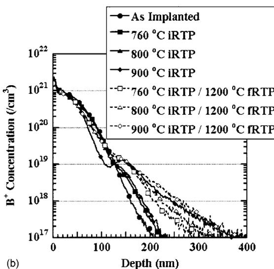
FIG. 3. Concentration profiles showing the  $B^+$  concentration as a function of depth for the 3-keV  $BF_2^+$  implant to  $6 \times 10^{14} \text{ cm}^{-2}$  before and after a 1200 °C fRTP for the (a) 48- and (b) 5-keV  $Ge^+$  preamorphization implants to  $5 \times 10^{14} \text{ cm}^{-2}$ . The symbols are for identification purposes only.
