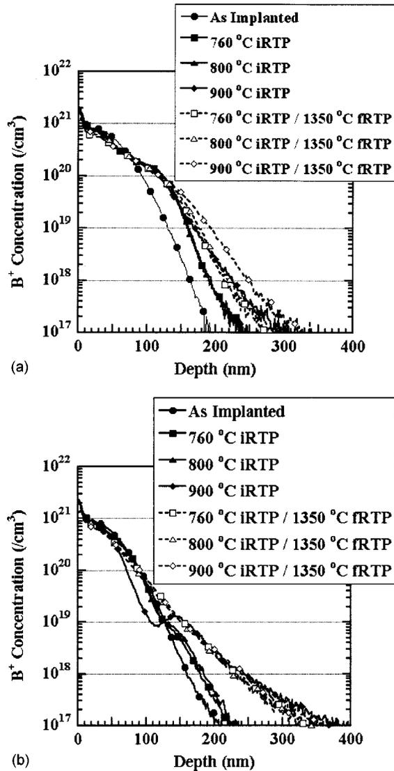
FIG. 4. Concentration profiles showing the  $B^+$  concentration as a function of depth for the 3-keV  $BF_2^+$  implant to  $6 \times 10^{14} \text{ cm}^{-2}$  before and after a  $1350^\circ\text{C}$  fRTP for the (a) 48- and (b) 5-keV  $Ge^+$  preamorphization implants to  $5 \times 10^{14} \text{ cm}^{-2}$ . The symbols are for identification purposes only.
