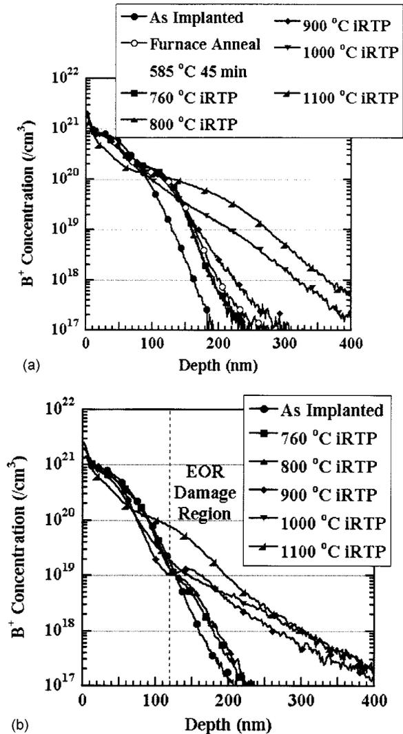
FIG. 2. Concentration profiles showing the  $\text{B}^+$  concentration as a function of depth for the 3-keV  $\text{BF}_3^+$  implant to  $6 \times 10^{14} \text{ cm}^{-2}$  after each iRTP anneal temperature used in this study for the (a) 48- and (b) 5-keV  $\text{Ge}^+$  preamorphization implants to  $5 \times 10^{14} \text{ cm}^{-2}$ . The symbols are for identification purposes only.
