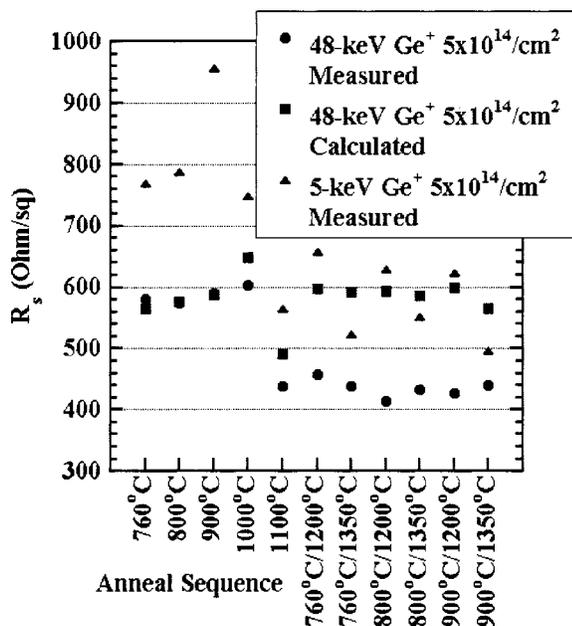
FIG. 6. Graph of the measured (●) and calculated (▲)  $R_s$  values obtained for the 48-keV  $\text{Ge}^+$  pre-amorphization implant to  $5 \times 10^{14} \text{ cm}^{-2}$  and the measured (○) values obtained for the 5-keV  $\text{Ge}^+$  preamorphization implant to  $5 \times 10^{14} \text{ cm}^{-2}$ .
