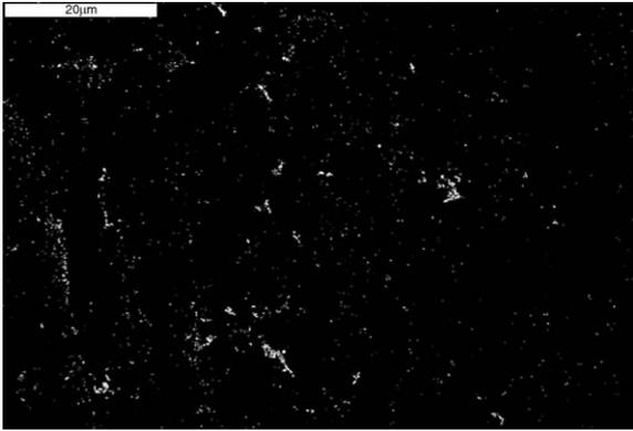
Fig. 2. NiO backscattered electron image; bright spots are metallic Ni particles.
