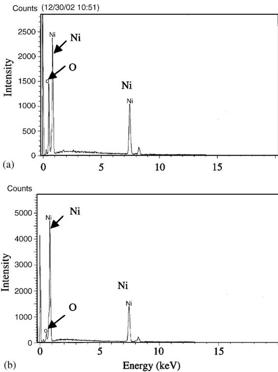
Fig. 3. EDS results of bright and dark regions in Fig. 2 (a) strong presence of oxygen in darker regions of Fig. 2, however (b) shows EDS spectrum of bright particle from Fig. 2 showing a lack of oxygen.
