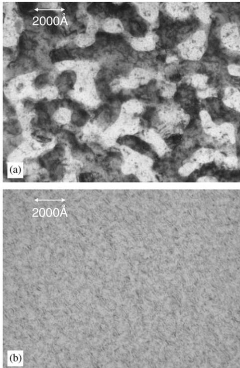
Fig. 5. Bright field TEM images of (a) NiO and (b) MnO fulgurites. NiO is clearly a two-phase mixture but the MnO fulgurite is a defective single phase.
