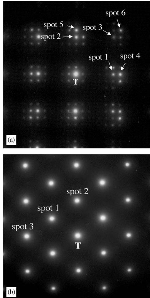
Fig. 6. Selected area diffraction pattern of fulgurites (a) NiO [001] zone axis (b) MnO [0–1 1] zone axis.
