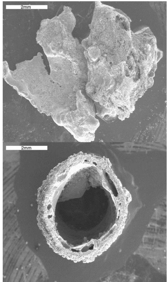
Fig. 1. Low-magnification SEM image of NiO fulgurite (top) and MnO fulgurite (bottom).
