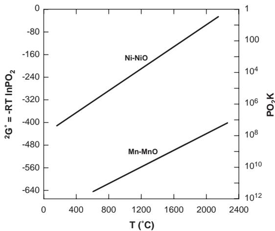
Fig. 8. Ellingham diagram of oxide stability at 1 at of oxygen. Note MnO is significantly more stable than NiO (DeHoff, 1993).
