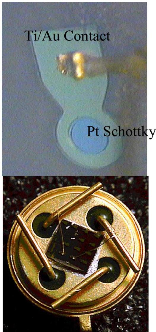
Fig. 2. SEM micrograph of completed device, showing bond wire attached (top) and photograph of device bonded into header.
