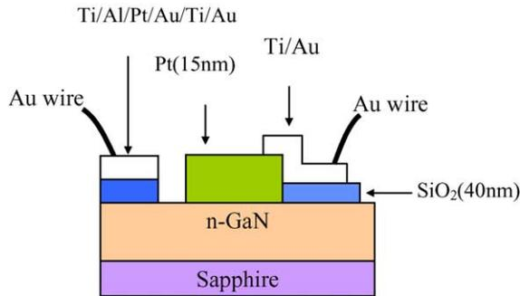
Fig. 1. Schematic of Pt/GaN Schottky diode for hydrogen gas sensing.
