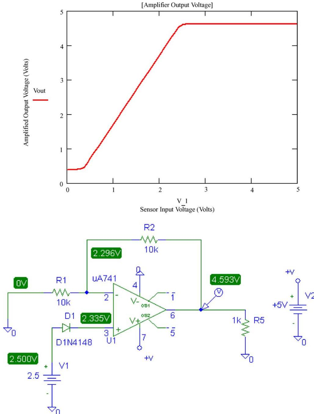
Fig. 4. Output of amplifier in response to change in sensor input voltage (top) and schematic of amplifier (bottom).
