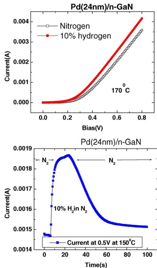
Fig. 3. Forward  $I$ - $V$  characteristics from Pt/GaN diode at 170 °C in either 10% H<sub>2</sub>/90% N<sub>2</sub> or pure N<sub>2</sub> ambient (top) and forward current at fixed bias of 0.5 V at 150 °C as a function of time as the ambient is switched from N<sub>2</sub> to 10% H<sub>2</sub>/90% N<sub>2</sub> (bottom).
