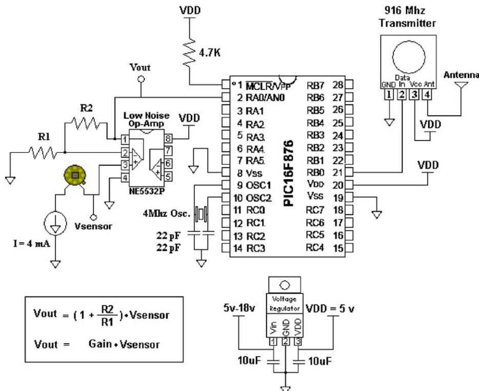
Fig. 5. Circuit diagram for transmitter sensor (top) and specifications (bottom).
