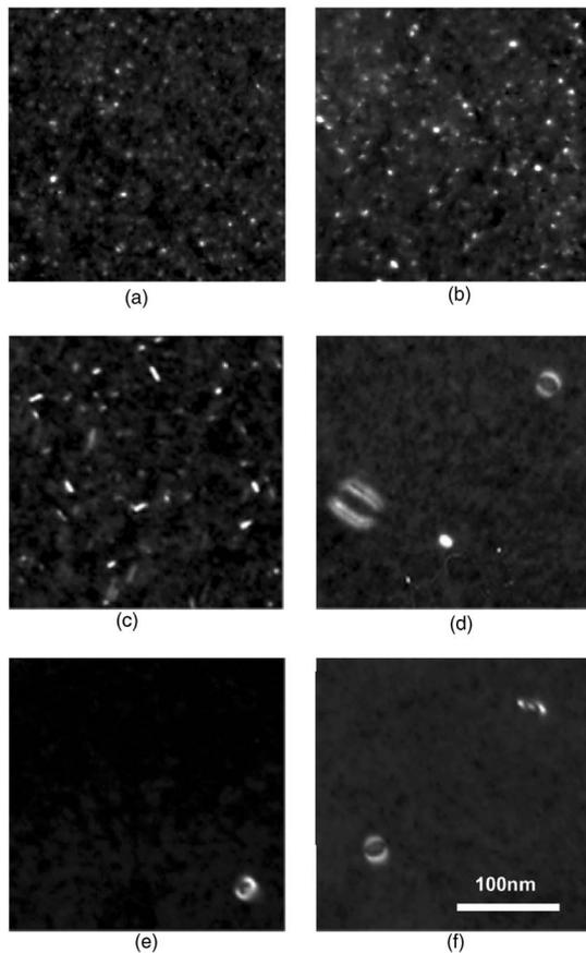
FIG. 1. WBDF PTEM images taken at  $g_{220}$  diffraction conditions of the end of range damage for the following anneal conditions: (a) 700 °C iRTP, 1000 °C fRTP, (b) 700 °C iRTP, 1100 °C fRTP, (c) 700 °C iRTP, 1200 °C fRTP, (d) 700 °C iRTP, 1300 °C fRTP, (e) 700 °C iRTP, 1100 °C fRTP + 950 °C RTA, and (f) 950 °C RTA only.
