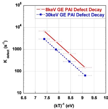
FIG. 4. (Color online) Arrhenius plot of the time constant derived for defect decay extracted from the simulated experimental data, indicating an activation energy  $E_a$  of  $2.2 \pm 0.05$  eV for dissolution.
