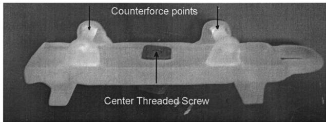
FIG. 1. Quartz apparatus used to create three-point bending in silicon samples. The counterforce points pin the silicon from the top and the screw applies an upward force resulting in a gradient radius of curvature in the silicon.
