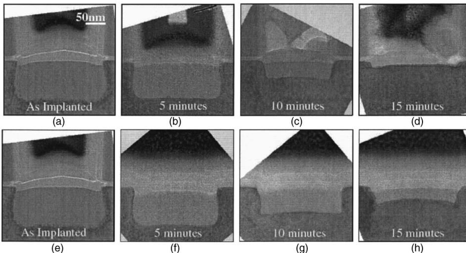
FIG. 3. XTEM partial recrystallization series at 550 °C. Images (a) and (e) are as implanted with the mask present. Images (b), (c), and (d) are material annealed with the mask present, and (f), (g), and (h) are material annealed after etching off the oxide-nitride mask. It is important to note the presence of the film and its associated tensile stress increases the corner velocity, thus preventing the apparent pinch point formation observed in the lower images without stress.
