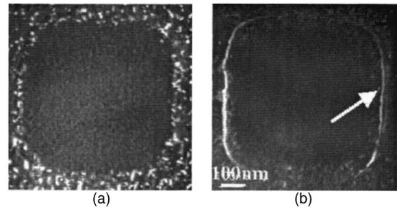
FIG. 2. PTEM showing the effect of removing the oxide-nitride implant mask on the formation of an edge defect after a 750 °C, 10 min anneal. The sample in (a) still has the mask present, while the sample in (b) has had the mask removed. The white arrow indicates the location of the edge defect (Ref. 1).
