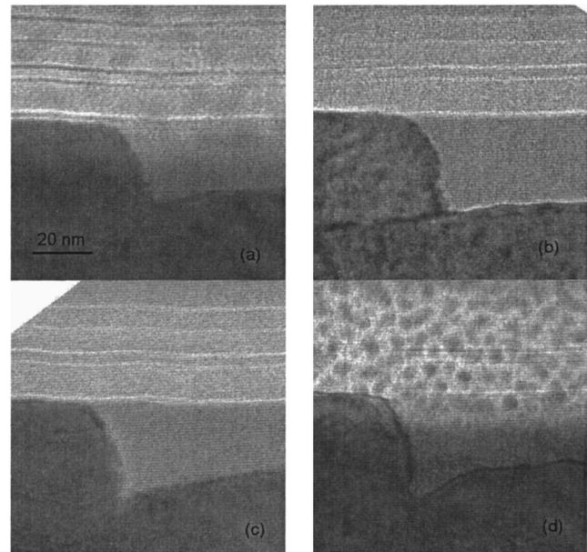
FIG. 5. XTEM of material to which (a) 50 MPa tension, (b) 100 MPa tension, (c) 50 MPa compression, and (d) 100 MPa compression have been applied while annealing at 550 °C for 13 min. It is observed that compression results in an acute angle at the corner of the amorphous-crystalline interface, while tension results in an obtuse angle.
