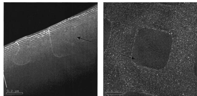
FIG. 6. PTEM after 550 °C, 1 h annealing at (a) 250 MPa compression or (b) 175 MPa tension. Note that there is no defect suppression for the compression case but a complete defect suppression in the tensile case.
