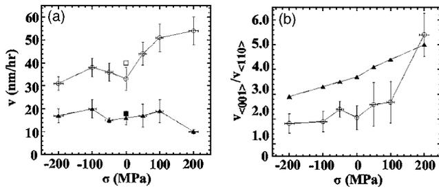
FIG. 4. Plots of (a)  $v_{(001)}$  (circles) and  $v_{(110)}$  (triangles) vs  $\sigma$  and of (b)  $v_{(001)}/v_{(110)}$ , observed (circles) and predicted (triangles), versus  $\sigma$ . The open (Ref. 11) and filled (Ref. 12) squares in (a) denote reported values of  $v_{(001)}$  and  $v_{(110)}$ , respectively.
