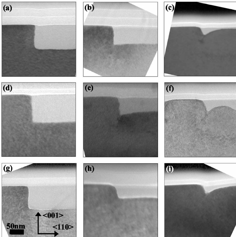
FIG. 2. XTEM micrographs of samples annealed for (a) 1 h, (b) 2 h, and (c) 3 h without stress; (d) 1 h, (e) 2 h, and (f) 3 h under compressive stress of 200 MPa; and (g) 1 h, (h) 2 h, and (i) 3 h under tensile stress of 200 MPa.
