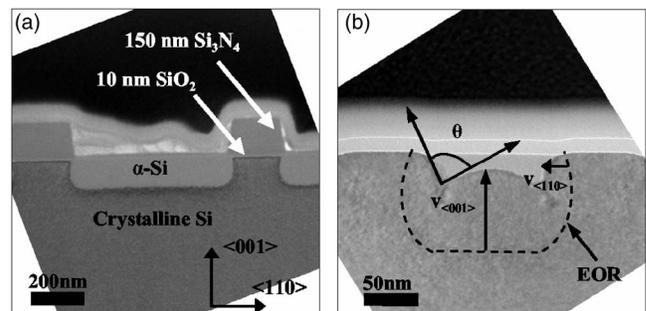
FIG. 1. XTEM micrographs of (a) an as-implanted structure and (b) schematic representations of the parameters  $\theta$ ,  $v_{\langle 001 \rangle}$ , and  $v_{\langle 110 \rangle}$ .
