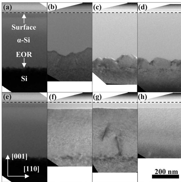
FIG. 1. [(a) and (e)] XTEM images of the as-implanted structure. XTEM images of specimens annealed for 7.0 h with applied stress of (b) -0.25 GPa, (c) -0.5 GPa, (d) -1.0 GPa, (f) 0, (g) 0.5 GPa, and (h) 1.0 GPa.
