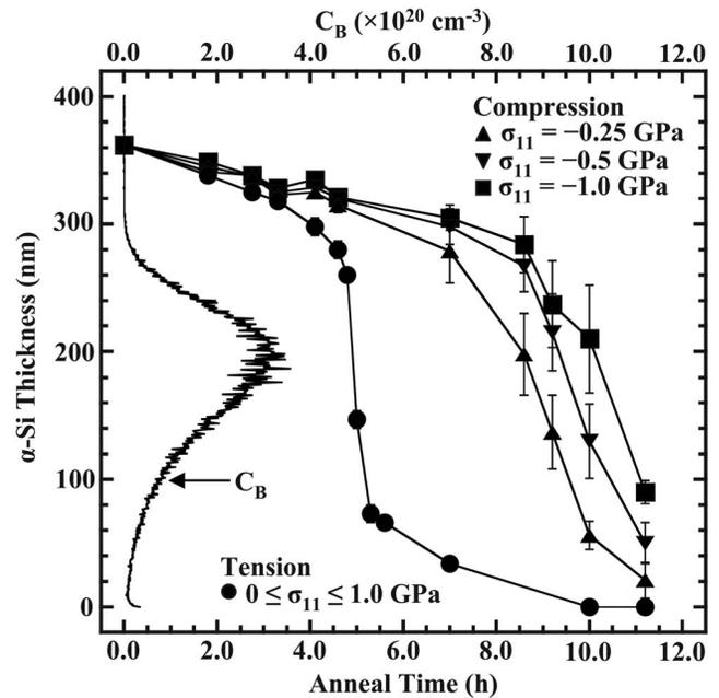
FIG. 2.  $\alpha$ -Si thickness versus anneal time behavior for different applied stress values ( $\sigma_{11}$ ) as superimposed on the SIMS-determined B concentration ( $C_B$ ) profile.
