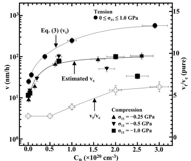
FIG. 3. Effect of B concentration ( $C_B$ ) on growth velocity ( $\nu$ ) for different applied stress values ( $\sigma_{11}$ ).
