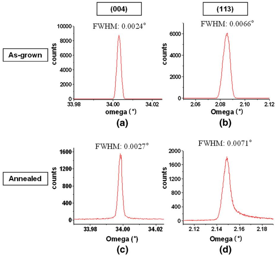
Fig. 2. (004) and (113) omega rocking curves (ω-RCs) acquired from the as-grown and annealed strained  $\text{Si}_{80}\text{Ge}_{20}$  layers.
