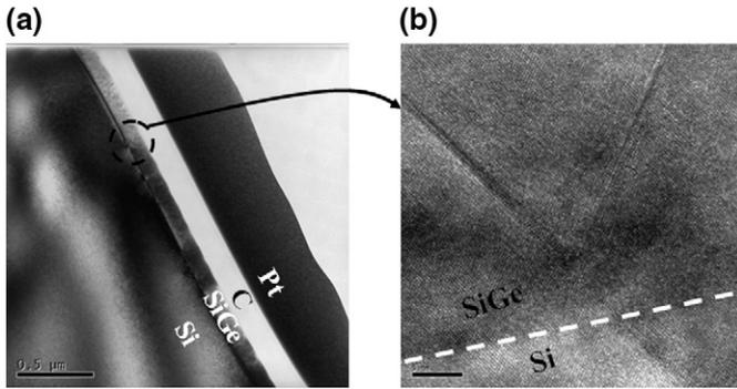
**Fig. 4.** (a) Cross-sectional and (b) high resolution TEM images in  $\langle 110 \rangle$  projection of 100 nm thick strained  $\text{Si}_{75}\text{Ge}_{25}$  annealed at  $900^\circ\text{C}$  for 30 min.
