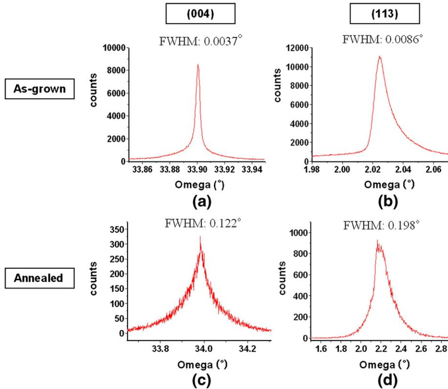
Fig. 3. (004) and (113) ω-RCs acquired from the as-grown and annealed at  $900^\circ\text{C}$  for 30 min  $\text{Si}_{75}\text{Ge}_{25}$  100 nm thick.
