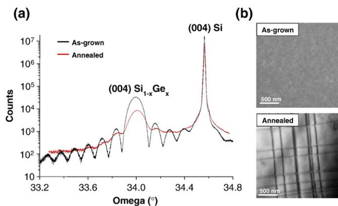
**Fig. 1.** (a) Omega-2theta rocking curves ( $\omega$ -2 $\theta$  RCs) and (b) plan-view transmission electron microscopy (PV-TEM) images of as-grown and annealed at  $800^\circ\text{C}$  for 30 min  $\text{Si}_{80}\text{Ge}_{20}$  films 50 nm thick.
