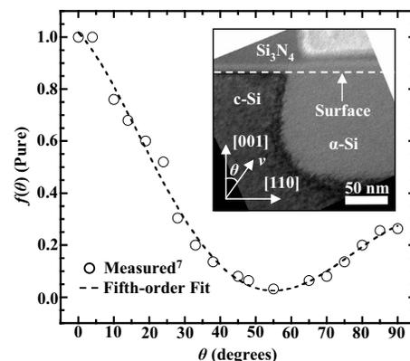
FIG. 1. The normalized SPER velocity,  $f(\theta)$ , as a function of the substrate orientation angle from [001] toward [110],  $\theta$ , as measured by Csepregi *et al.* (Ref. 7) The inset shows an XTEM micrograph of a typical 2D structure where the SPER process occurs.
