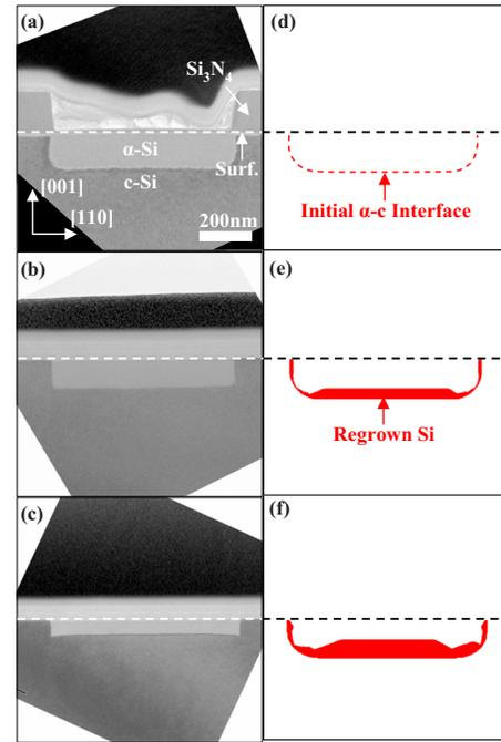
FIG. 2. (Color online) The observed and curvature-free simulated 2D SPER process in a structure with  $\alpha$ - $c$  interfacial pinning at the surface at  $T = 500^\circ\text{C}$ : XTEM images of the structure (a) as-implanted, (b) after 1 h of annealing, and (c) after 2 h of annealing. Level set simulations of the structure evolution using only regrowth orientation dependence [Eq. (1)] (d) as-implanted, (e) after 1 h of annealing, and (f) after 2 h of annealing.
