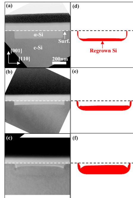
FIG. 3. (Color online) The observed and curvature-included simulated 2D SPER process in a structure with  $\alpha$ - $c$  interfacial pinning at the surface at  $T=500\text{ }^\circ\text{C}$ : XTEM images of the structure after annealing for (a) 1, (b) 2, and (c) 4 h. Level set simulations of the structure evolution using both regrowth orientation and interfacial curvature dependence [Eq. (2)] for (d) 1, (e) 2, and (f) 4 h.
