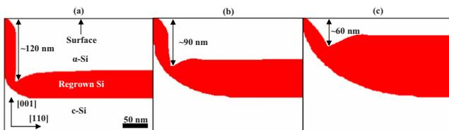
FIG. 5. (Color online) The effect of initial  $\alpha$ - $c$  interface curvature near the corner region on the level set simulations using both regrowth orientation and interfacial curvature dependence [Eq. (2)] of the 2D SPER process in a structure with  $\alpha$ - $c$  interfacial pinning at the surface:  $r=(a)$  40, (b) 80, and (c) 120 nm.
