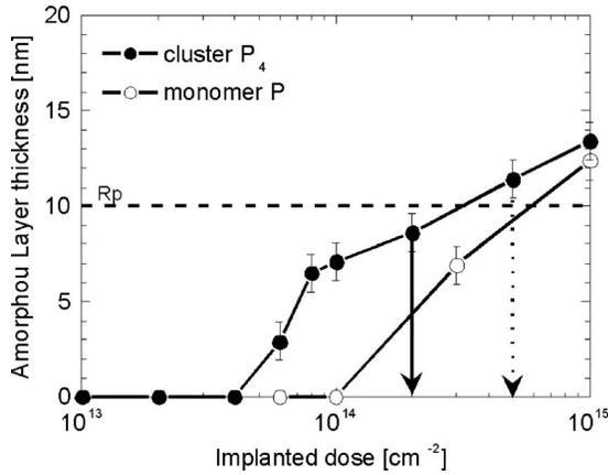
FIG. 2. Amorphous layer thickness measured by TEM in 5 keV  $P_4^+$  cluster (full symbols) and monomer (empty symbols) implanted samples vs implanted dose. The solid line arrow indicates the formation of continuous amorphous layer by cluster ion implantation measured in this work. Amorphization threshold by monomer ion implantation (dotted line arrow) is also indicated. 5 keV P projected ranges is indicated.
