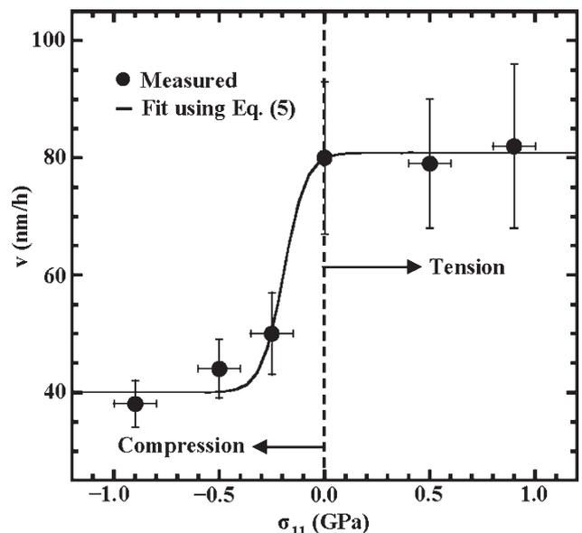
FIG. 3. Plot of the time-averaged (011)-oriented growth velocity ( $v$ ) at 525 °C versus applied in-plane  $[2\bar{1}1]$  uniaxial stress ( $\sigma_{11}$ ).
