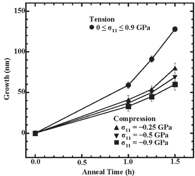
FIG. 2. Plot of (011)-oriented growth (epitaxial crystallization of amorphous Si) versus anneal time behavior at 525 °C for different applied in-plane  $[2\bar{1}1]$  uniaxial stresses ( $\sigma_{11}$ ).
