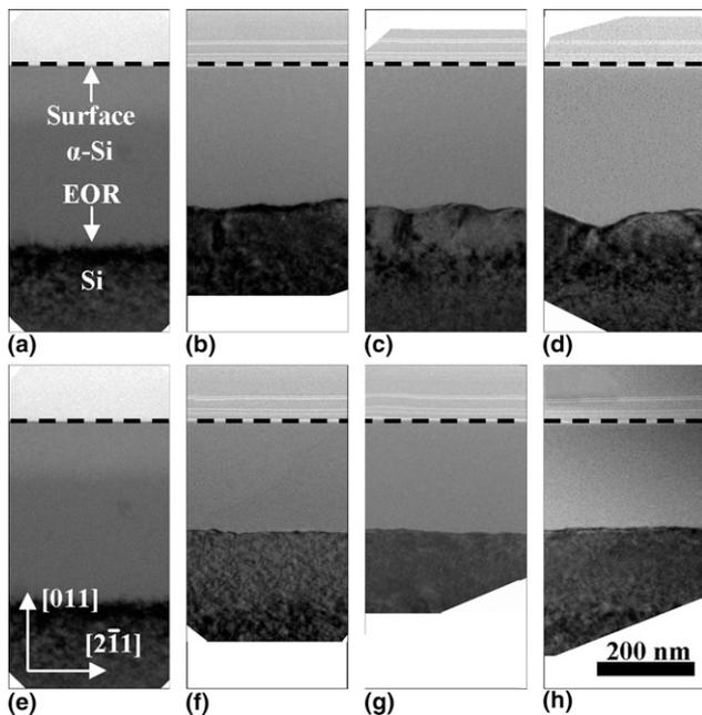
FIG. 1. (a, e) XTEM images of the as-implanted structure. XTEM images of specimens annealed for 1.5 h at 525 °C with applied in-plane  $[2\bar{1}1]$  uniaxial stress of (b)  $-0.25$ , (c)  $-0.5$ , (d)  $-0.9$ , (f)  $0$ , (g)  $0.5$ , and (h)  $0.9$  GPa.
