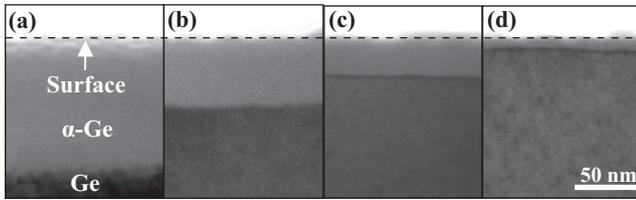
**Fig. 1.** XTEM micrographs of the solid-phase epitaxial growth process at 330 °C of (0 0 1) Ge self-implanted at 90 keV to a dose of  $2.0 \times 10^{15} \text{ cm}^{-2}$ : (a) the as-implanted structure, (b) after annealing for 44 min, (c) after annealing for 88 min, and (d) after annealing for 132 min.
