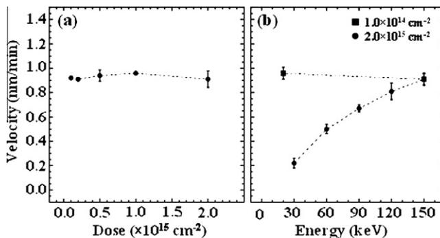
**Fig. 3.** The solid-phase epitaxial growth velocity at 330 °C of self-implanted (0 0 1) Ge: (a) the effect of implanted dose for samples implanted at 150 keV and (b) the effect of implant energy for samples implanted at a dose of  $1.0 \times 10^{14}$  or  $2.0 \times 10^{15} \text{ cm}^{-2}$ .
