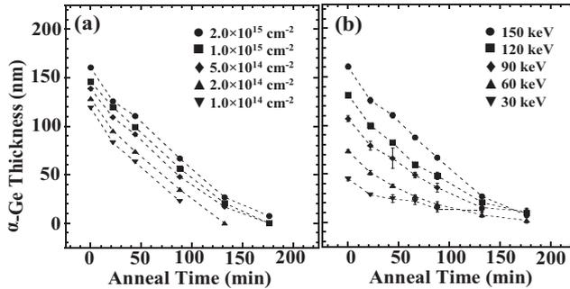
**Fig. 2.** Amorphous layer thickness versus annealing time behavior at 330 °C of self-implanted (0 0 1) Ge: (a) samples implanted at 150 keV with doses of  $1.0 \times 10^{14}$ – $2.0 \times 10^{15} \text{ cm}^{-2}$  and (b) samples implanted with energies of 30–150 keV with a dose of  $2.0 \times 10^{15} \text{ cm}^{-2}$ .
