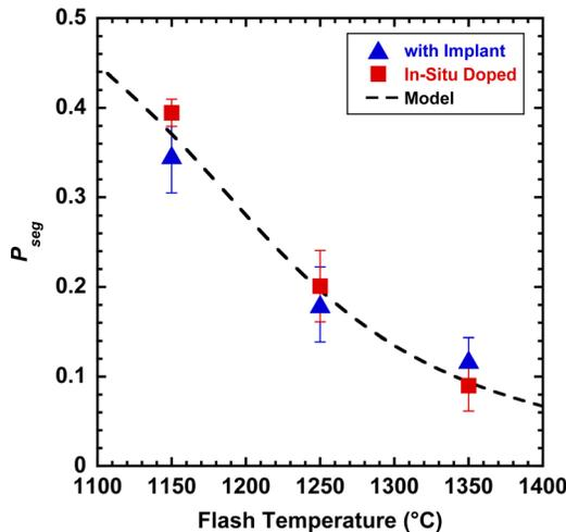
FIG. 4. (Color online)  $p_{seg}$  values from atom probe tomography are plotted for both the *in situ* doped (squares) and implanted (triangles) samples. The dotted line represents the values generated from the model.
