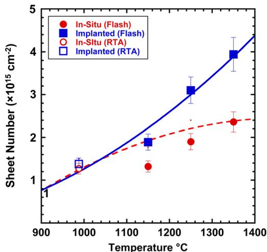
FIG. 6. (Color online) Sheet number values from Hall measurements for *in situ* doped and implanted samples annealed using flash and conventional RTA. Dashed and solid lines represent the theoretical activation for *in situ* doped and implanted samples, respectively.
