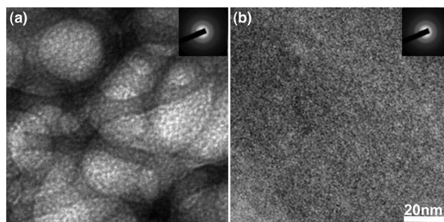
FIG. 4. HR-XTEM images (inset SAED patterns) showing the morphological evolution of nanostructured Ge electrodes with electrochemical cycling at a  $C/7.2$  rate: (a) an untested electrode and (b) an electrode after 25 cycles.
