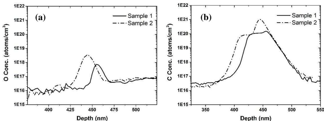
Figure 1. As-grown SIMS profiles of interfacial oxygen (a) and carbon (b) peaks for GaAs on Si samples with varied pre-clean. Sample 2 exhibits greater oxygen and carbon peak concentrations, indicating a larger amount of interfacial contamination. Peaks positions are offset based on layer thickness as determined by XTEM.
