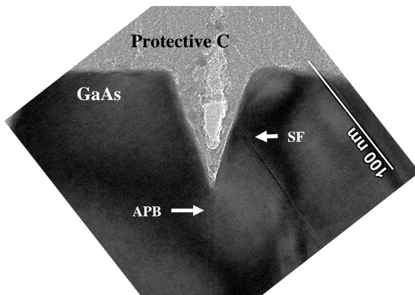
Figure 3. XTEM of etch pit in Sample 2 formed by HF/HNO<sub>3</sub> stain showing selectivity of etching for APB. Other defects, such as a stacking fault (SF) visible in the image, are not as reactive with the solution over the time scale of the etch.
