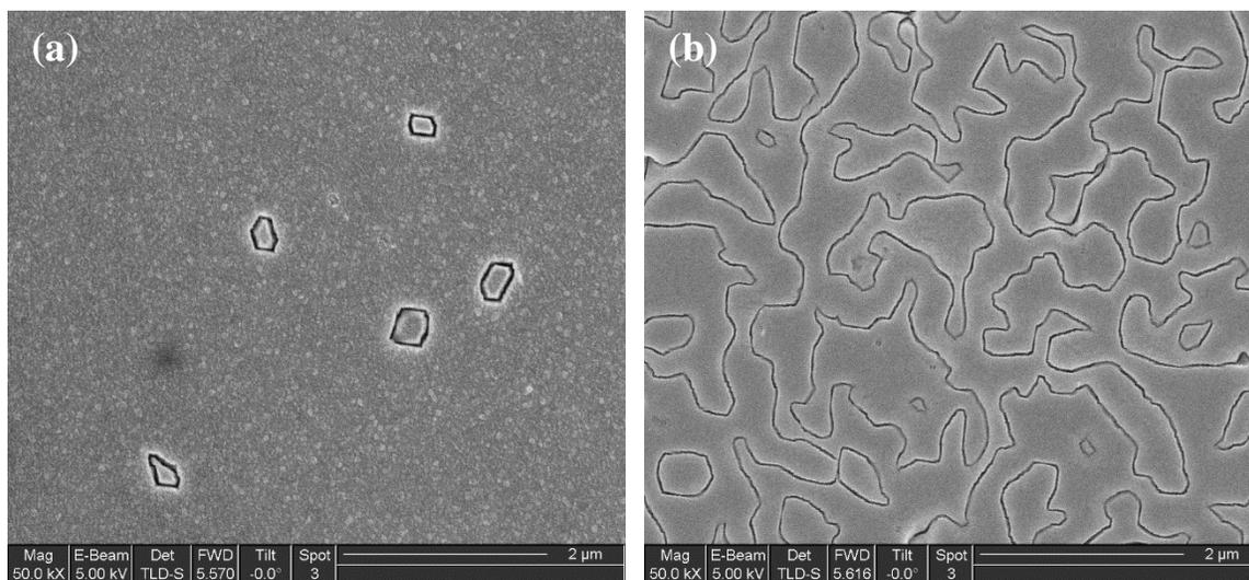
Figure 2. Plan-view SEM images of Sample 1 with lower oxygen and carbon interfacial dose (a) and Sample 2 with higher oxygen and carbon interfacial dose (b) after application of HF/HNO<sub>3</sub> chemical stain. APBs are clearly visible as features of dark contrast. The APB density dramatically increases with an approximately 5-10x increase in oxygen and carbon interfacial dose.
