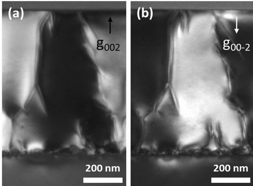
**Fig. 4.** Dark field-XTEM images of an APD in the sample with bulk layer grown at 630 °C using (002) (a) and (00-2) (b) reflections. The reversal of contrast within the APD relative to the surrounding crystal from (a) to (b) demonstrates this is an APD.
