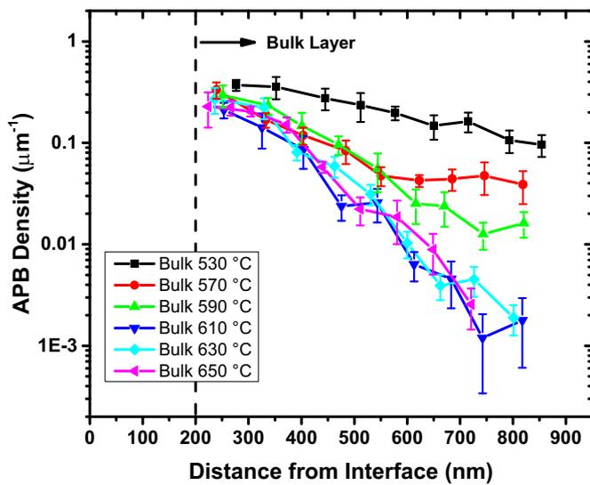
**Fig. 2.** Plot of through-thickness APB density for all GaAs-on-Si samples with varied bulk layer growth temperature. APB density decreases during growth due to APB kinking and annihilation. The annihilation rate with respect to film thickness is enhanced by increasing the bulk layer temperature up to 610 °C.
