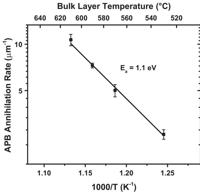
**Fig. 6.** Arrhenius plot of APB annihilation rate versus inverse bulk layer growth temperature. The activation energy was found to be 1.1 eV. This energy is representative of the barrier for APBs kinking to higher-index planes and annihilating.
