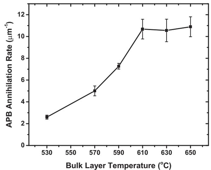
**Fig. 3.** Plot of APB annihilation rate with respect to film thickness for all samples versus bulk layer growth temperature. Annihilation rate increases with increasing temperature until saturation at 610 °C.
