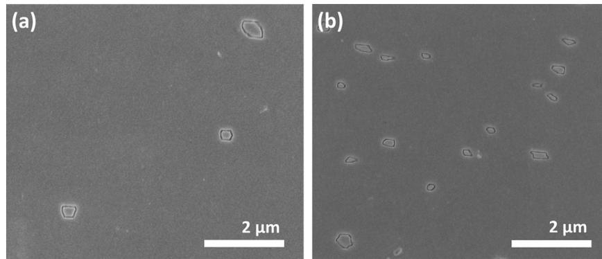
**Fig. 1.** Plan view SEM images of sample grown with a bulk layer at 570 °C at a film thickness of 745 nm (a) and 240 nm (b). The corresponding APB densities for these specimens are  $0.047 \pm 0.017 \mu\text{m}^{-1}$  (a) and  $0.33 \pm 0.06 \mu\text{m}^{-1}$  (b). There is a clear decrease in the number of antiphase domains with increasing film thickness. The specimens were stained with the HF/HNO<sub>3</sub> solution to improve APB contrast.
