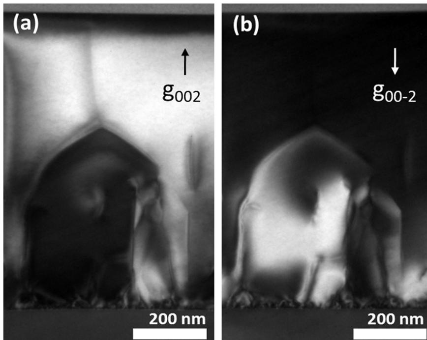
**Fig. 5.** Dark field-XTEM images of the sample with bulk layer grown at 610 °C using (002) (a) and (00-2) (b) reflections showing an APD terminating within the GaAs layer. The angle of APB annihilation is consistent with {112} type planes.
