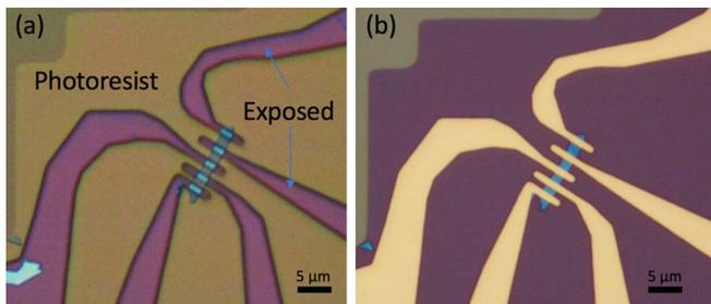
**Figure 4.** Optical microscope images depicting the process flow for contact-region implanted samples. Photolithographic patterning was used to define the device channels (a). Implantation was performed after (a) and prior to metal contact deposition, with the photoresist protecting the channel during implantation. (b) depicts a typical completed device on a few-layer MoS<sub>2</sub> flake.
