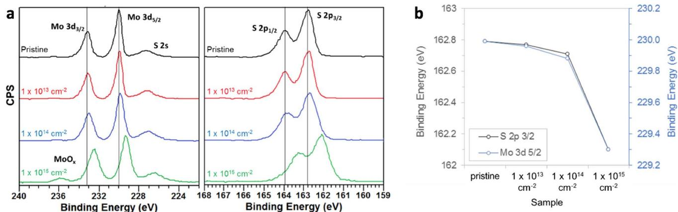
**Figure 1.** (a) XPS analysis of the pristine and implanted bulk mineralogical MoS<sub>2</sub> shows broadening of the peaks and (b) decreasing binding energy with increasing Cl<sup>+</sup> dose.
