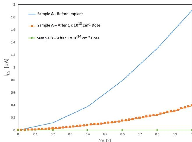
**Figure 5.** Output characteristics for before and after implantation of the channel with a  $1 \times 10^{13} \text{ cm}^{-2}$  dose of Cl (Sample A), and a typical high resistance result after implantation of the channel with  $1 \times 10^{14} \text{ cm}^{-2}$  dose of Cl (Sample B). A nearly 5 $\times$  reduction in current is observed after implantation of the channel with a  $1 \times 10^{13} \text{ cm}^{-2}$  dose of Cl (Sample A).
