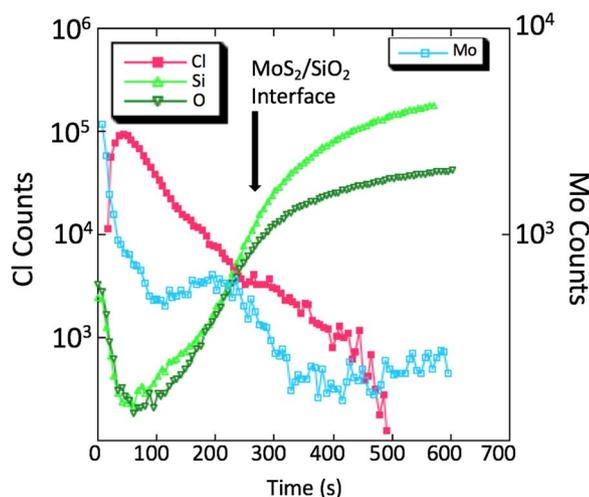
**Figure 2.** SIMS results for a 3–5 layer-thick grown MoS<sub>2</sub> film on SiO<sub>2</sub> after implantation with a 1 × 10<sup>13</sup> cm<sup>-2</sup> dose of Cl at an implant energy of 200 eV, confirming implantation into the top layers of the MoS<sub>2</sub>.
