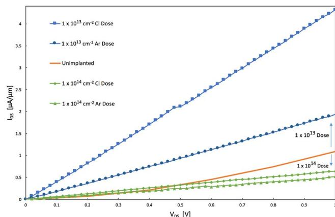
**Figure 6.** Output characteristics of contact-region implanted MoS<sub>2</sub> devices with a channel length of 1  $\mu\text{m}$ .
