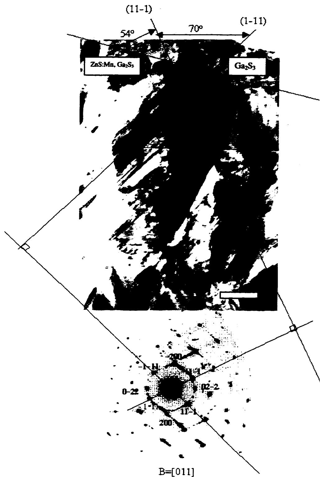
Figure 5.7 Bright field image and diffraction taken from sample with \text{Ga}_2\text{S}_3 after 5 minutes of annealing at 800^\circ\text{C} . (Bar = 100nm)
